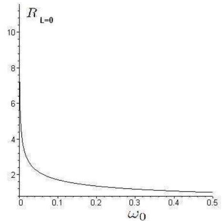
**Fig. 3** The  $(2\omega_0)^{-1/3}$  curve, where  $L^2 = 0$ . Stable circular orbits exist for radii lying above this curve.
