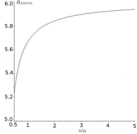
**Fig. 2** The ISCO radius as a function of the dimensionless parameter  $\omega_0$  in the black hole regime. For large  $\omega_0$  values the radius of the ISCO is approaching  $R_{ISCO} = 6$  which is the Schwarzschild case.
