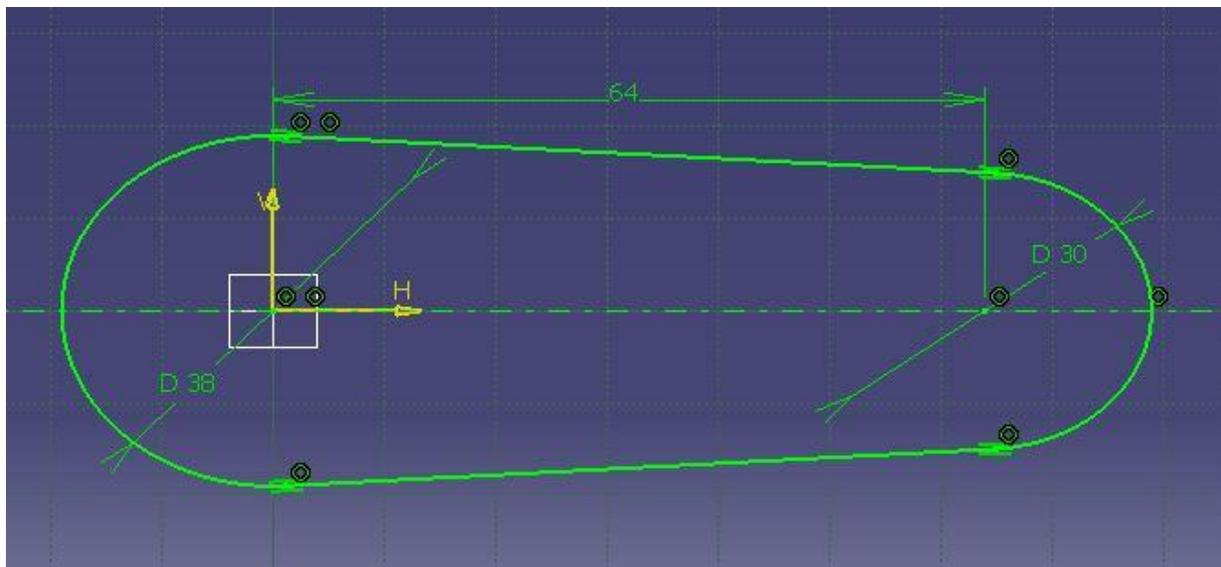
Select Sketch.1 as the profile to be extruded. Click Pad
