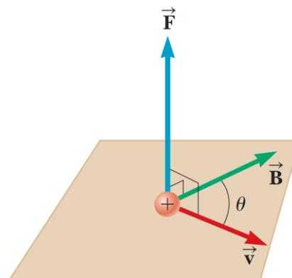
Figure 1. Direction of the force exerted by a magnetic field on a moving charged particle
