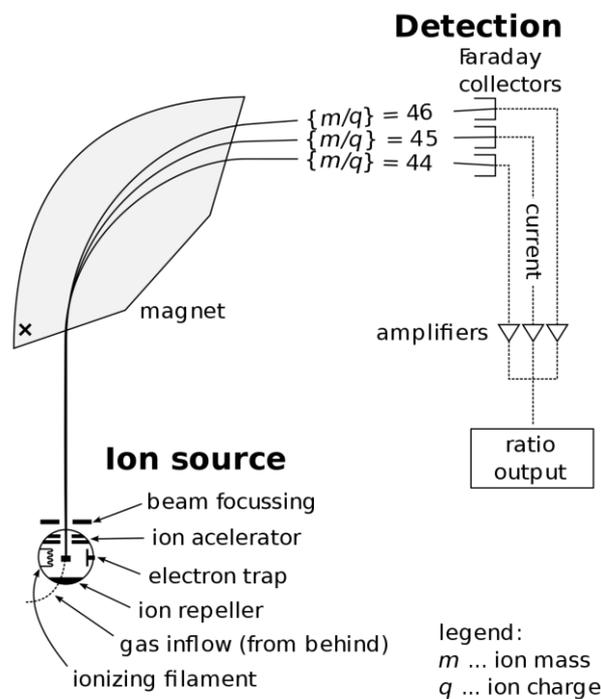
Figure 2. Setup of a mass spectrometer (source: wikipedia)
