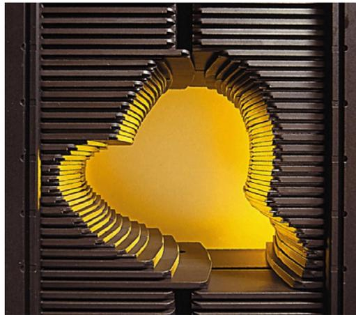
Figure 2: multi-leaf collimator<sup>1</sup>
