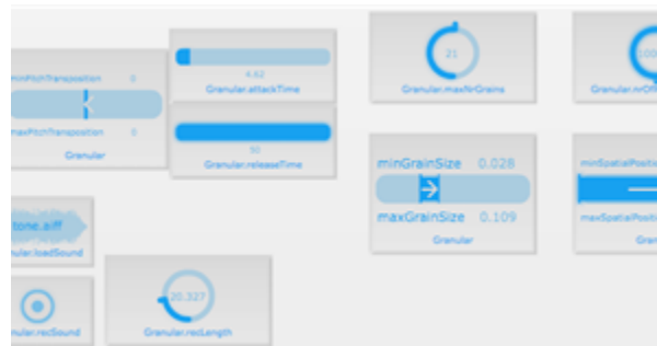
Figure 11.1. A granular synthesizer in Live View. It can process either pre-recorded sounds (stored in Granular.loadSound ) or live input (which can be recorded with Granular.recSound ).
