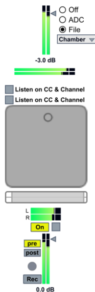
Figure 14.3. A simple stereo panner in Max. The 2D interface controls both the stereo positioning and depth.
