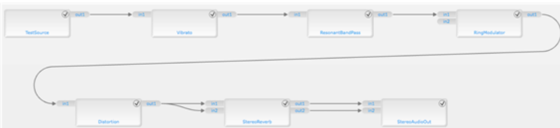
Figure 15.1. A block consisting of a test tone, modulated, filtered and distorted in several ways.
