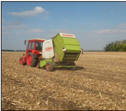
FIGURE 1: CLAAS ROLLANT 66 Round baler (fix chamber)
