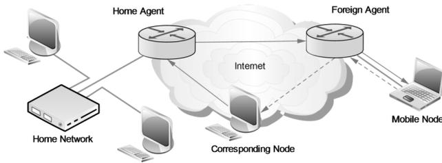
Fig. 1. IPv4 mobility packet routing
