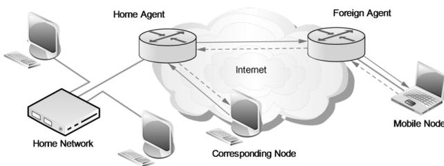
Fig. 2. IPv4 mobility reverse tunneling
