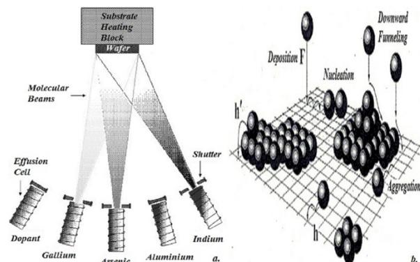
Figure 1. The structure of the MBE instrument (a.) and the process of the layer growth (b.) (source: [5]).
