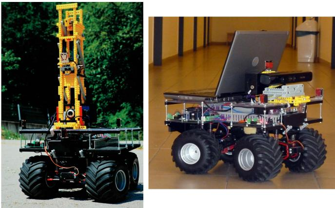
Fig. 1. Our mobile robot system with laser based sensor to the left [1], and with Kinect sensor to the right [2].
