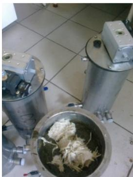
Figure 3: Batch anaerobic digestion with pre-treated chicken feather
