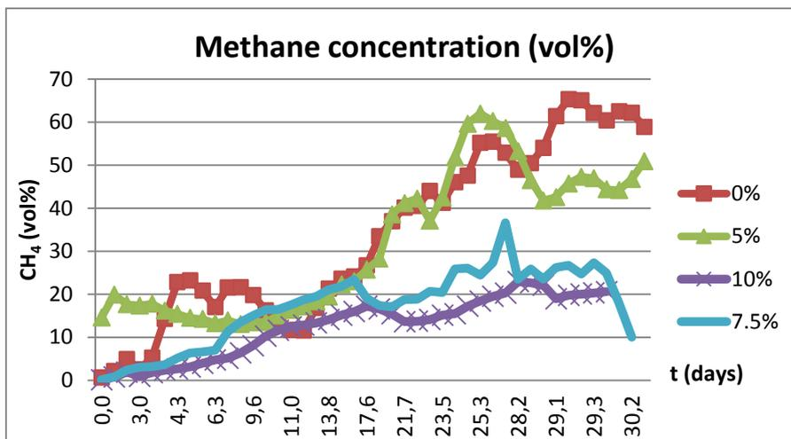
Chart 2: Methane concentration (vol%) production during co-digestion of different pre-treated feather ratio
