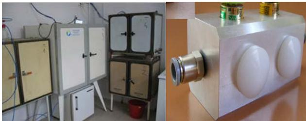
Figure 1: Incubators and custom created biogas analyser
