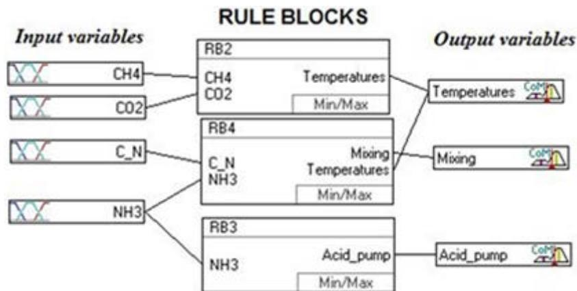
Figure 4: Adaptive fuzzy control of the biogas process
