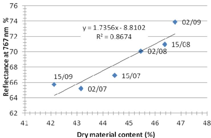
**Figure 2.** Correlation between reflectance at a specified spectrum with dry material content
