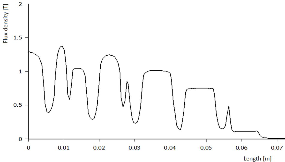
Fig. 4. Flux Density in the Machine Air-Gap
