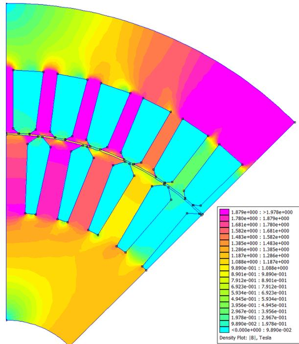
Fig. 3. Flux Density Distribution
