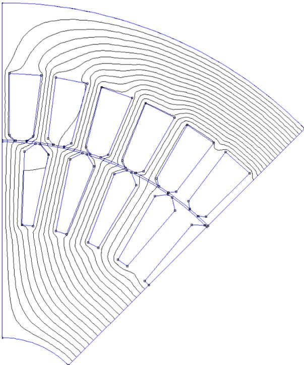
Fig. 2. Magnetic Potential Distribution
