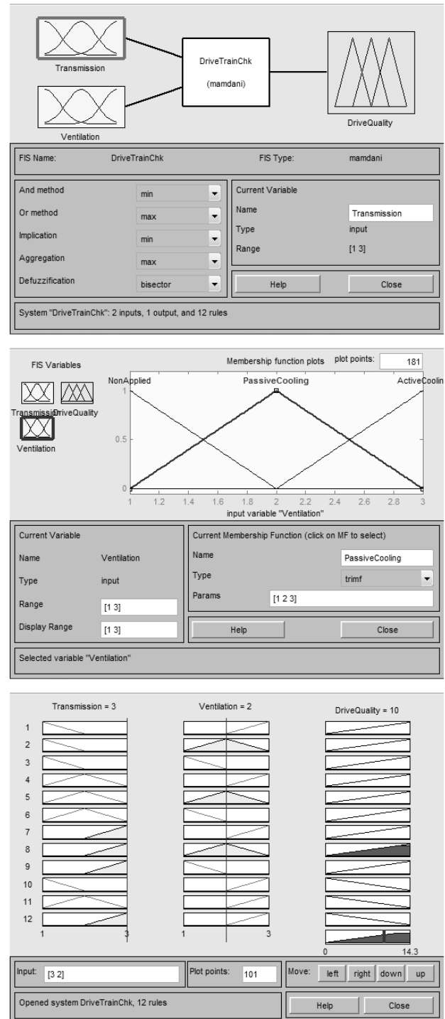
Figure 1 Typical fuzzy inference system in MATLAB environment with fuzzy membership functions in the input range and rules among the membership functions.
