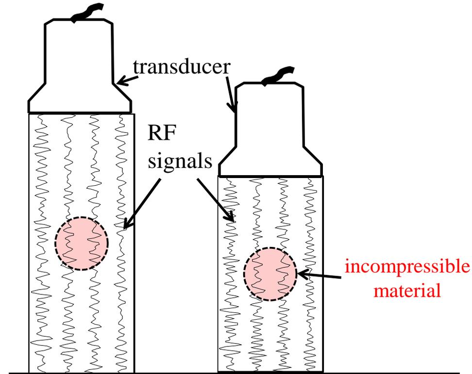
Quasi-static elastography schematic. Incompressible red inclusion is detected by taking cross-correlations between A-line segments before and after compression and finding no relative displacement inside inclusion. Figure adapted from [Konofagou 2004].
