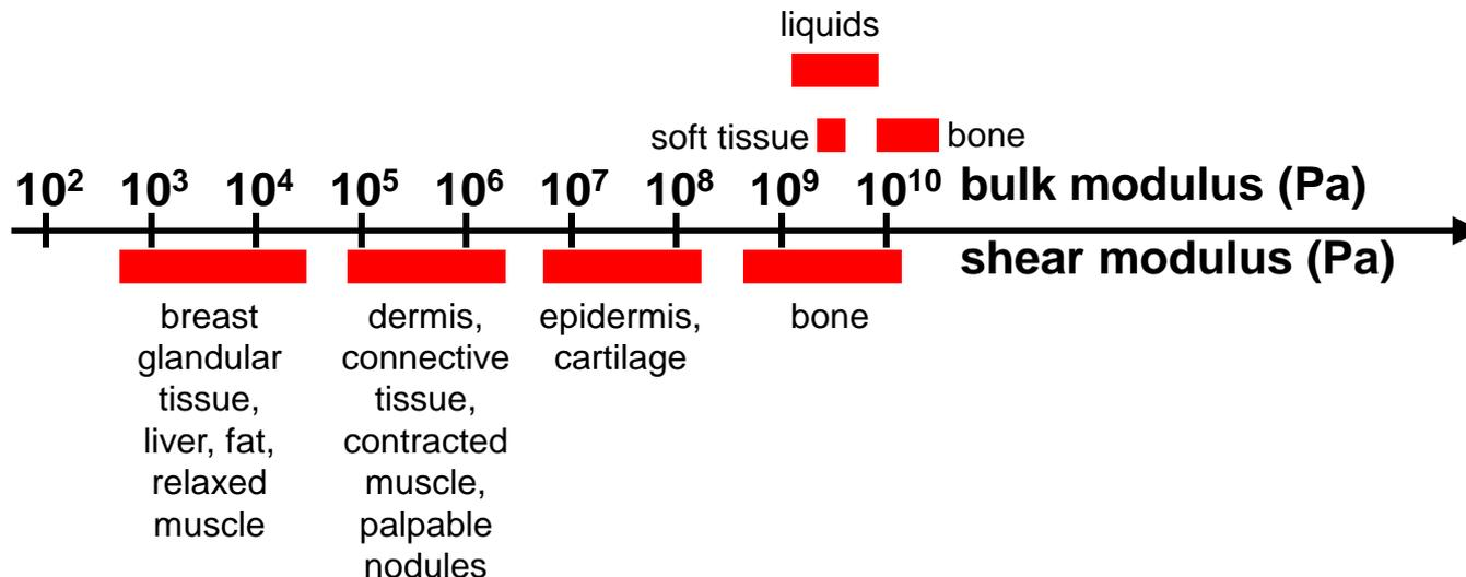
Comparison of shear and bulk moduli. Adapted from [Sarvazyan *et al.* 1998].
