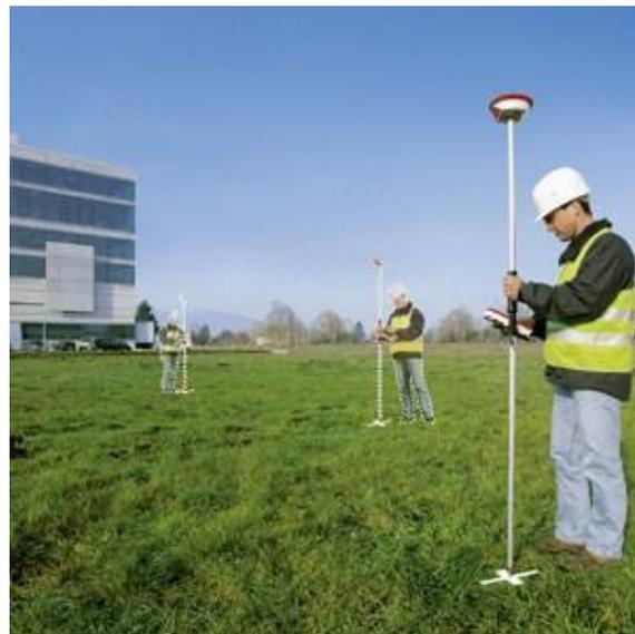
Figure 5. GPS rover instrument
