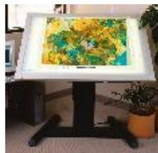
Figure 13. Large format backlit digitizing table
