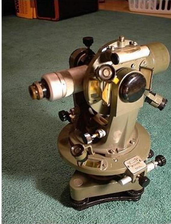
Figure 10. The soviet optical theodolite built in 1958
