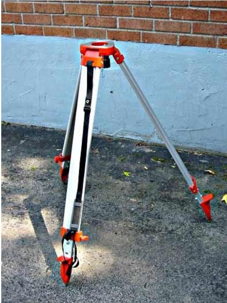
Figure 11. The surveyor's tripod
