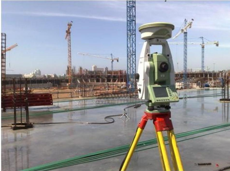
Figure 13. The robotic total station with GPS receiver equipped
