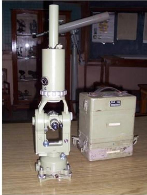
Figure 15. Upper mounted gyrotheodolite
