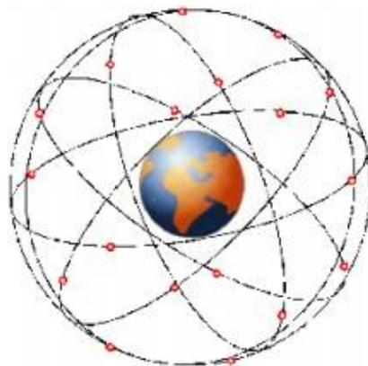
Figure 3-2.: The six orbit planes of GPS
