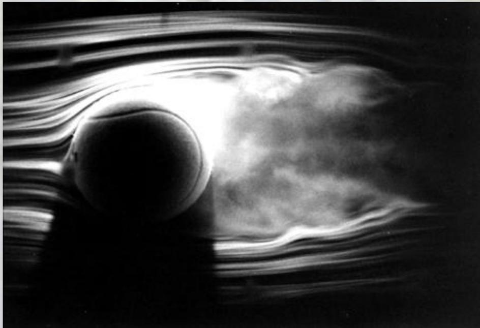
The laminar flow trajectories are around the ball, the eddies can be found before it
