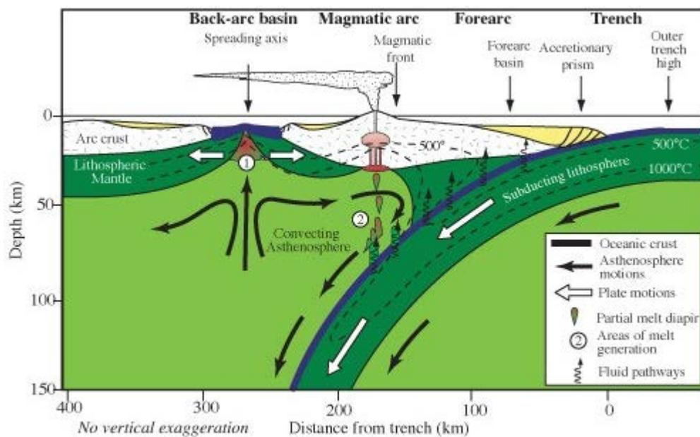
*Cross section of a subduction zone showing the situation of fore-arc and back-arc basins [iv]*
