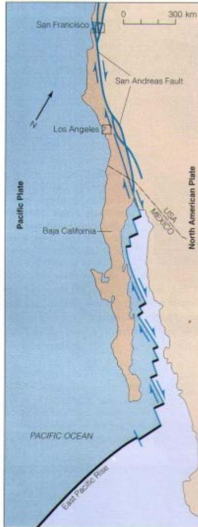
***The San Andreas Fault as a typical example of a transform fault plate margin [ix]***
