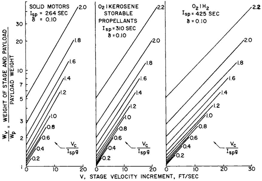
Fig. 2 Weight-velocity profiles for rocket stages
