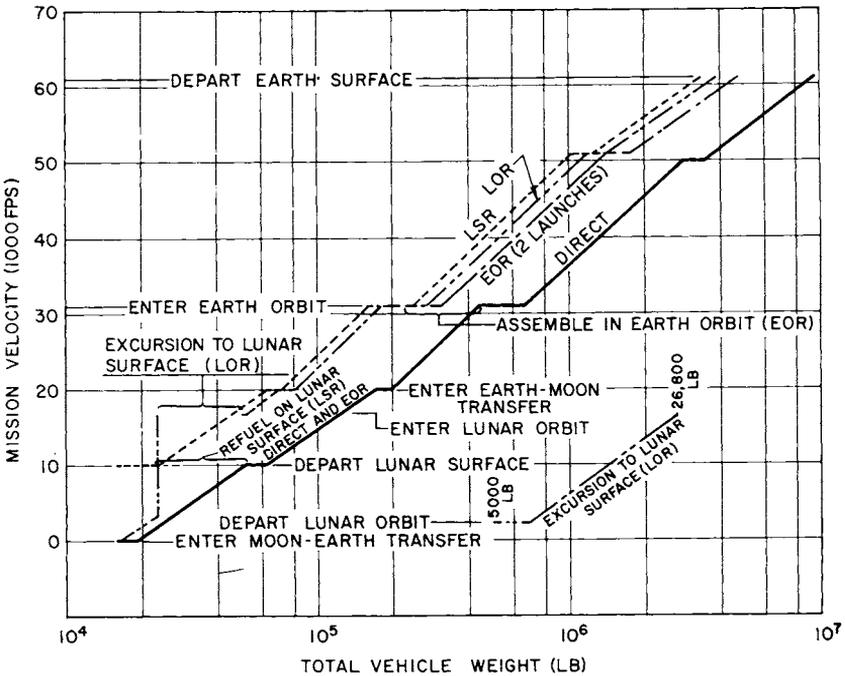
Fig. 7 Weight-velocity profiles - comparison of mission plans
