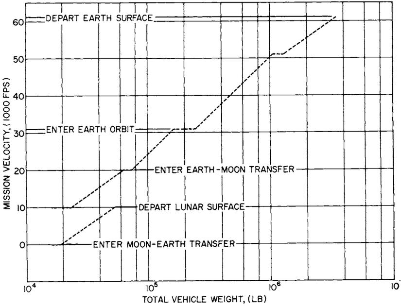
Fig. 6 Weight-velocity profile - lunar surface rendezvous
