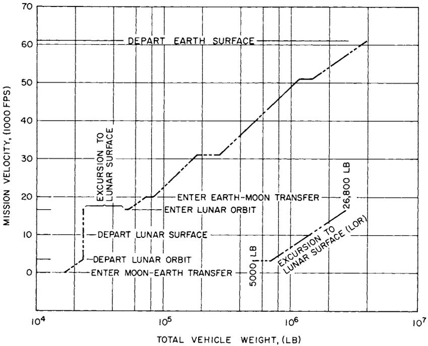
Fig. 5 Weight-velocity profile - lunar orbit rendezvous
