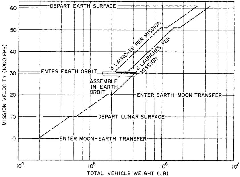
Fig. 4 Weight-velocity profile - earth orbit rendezvous
