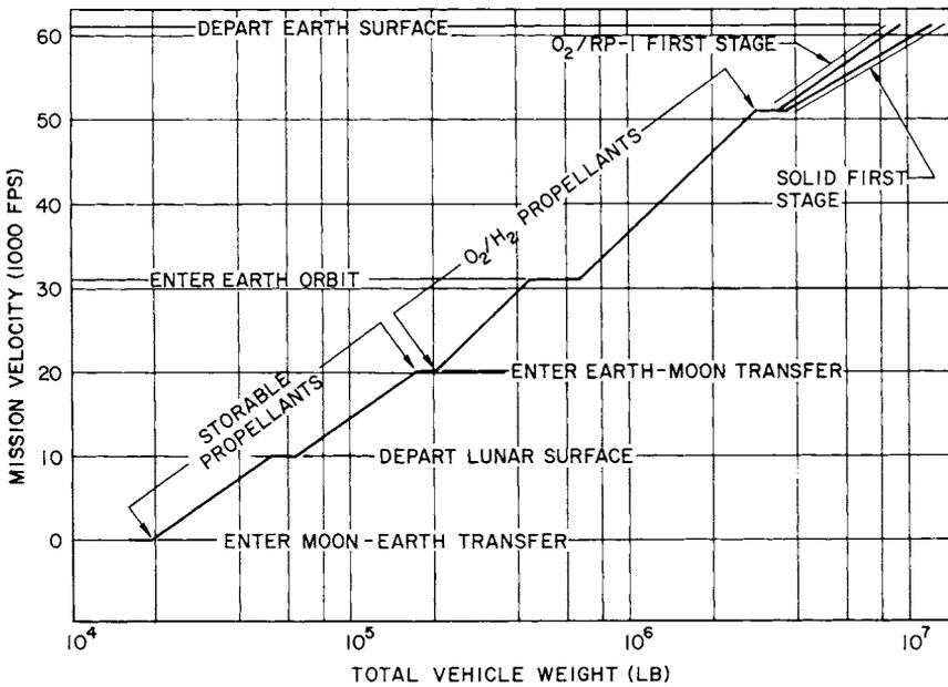
Fig. 3 Weight-velocity profile - direct lunar mission
