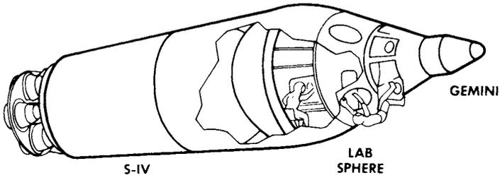
Fig. 4 Saturn S-IV Stage Intermediate Orbit Manned Space Station
