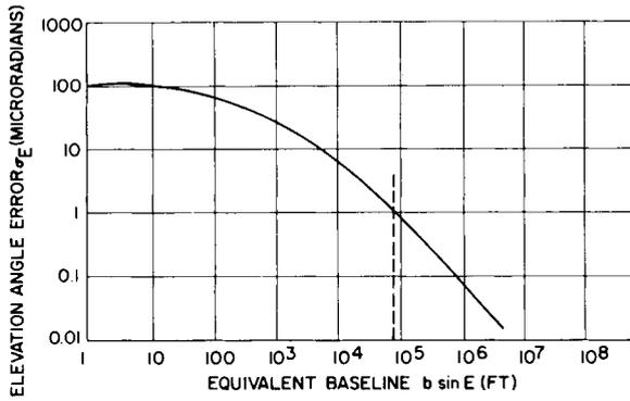
Fig. 4 Angle measurement errors caused by propagation
