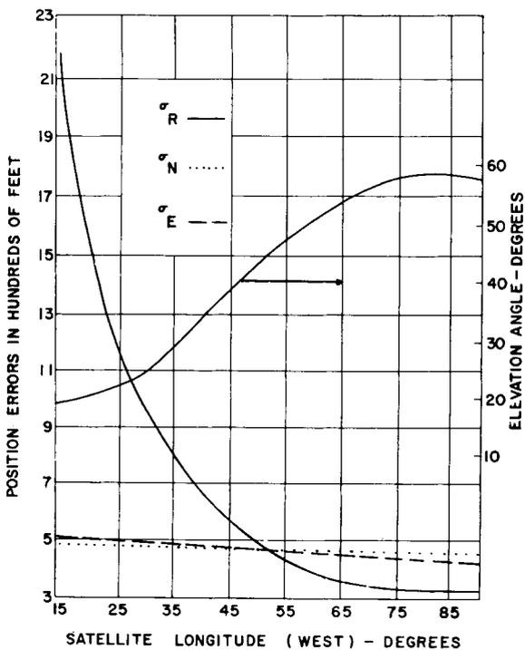
Fig. 9 Position errors - synchronous satellite
