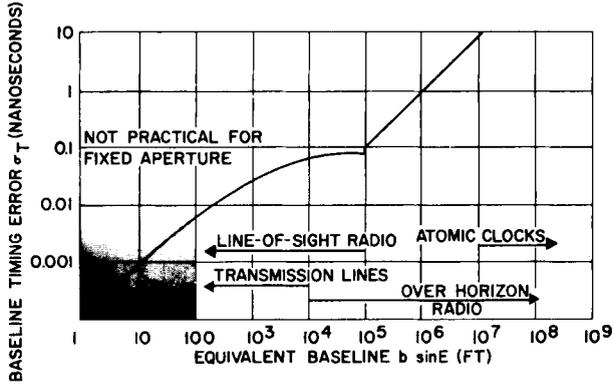
Fig. 6 Allowable timing errors
