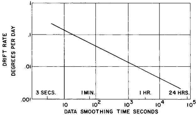
Fig. 11 Apparent drift rate of synchronous satellite as function of data smoothing time
