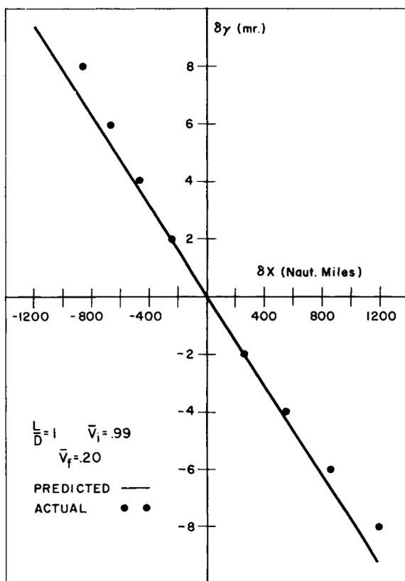
Fig. 4 Comparison between predicted and actual range deviation due to nonequilibrium glide initial condition in flight path angle
