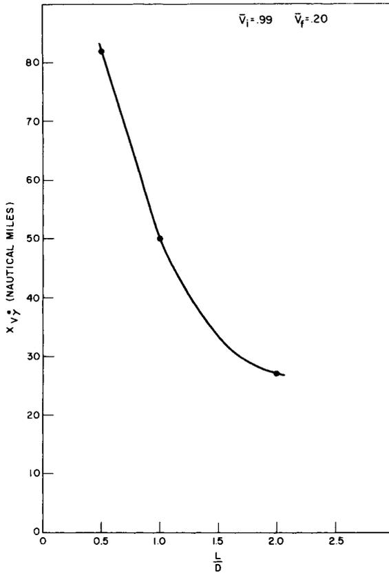
Fig. 6 Range associated with  $\bar{V}_\gamma$  as a function of L/D
