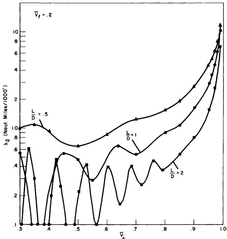
Fig. 3 Range deviation due to nonequilibrium glide initial condition in altitude
