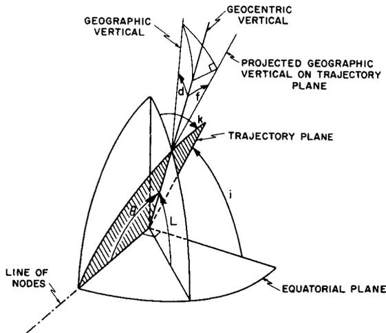
Fig. 7 Quantities required for analysis of two-dimensional trajectory on a nonspherical planet
