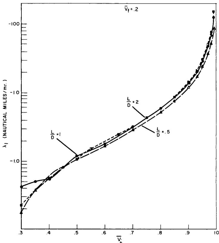
Fig. 2 Range deviation due to nonequilibrium glide initial condition in flight path angle
