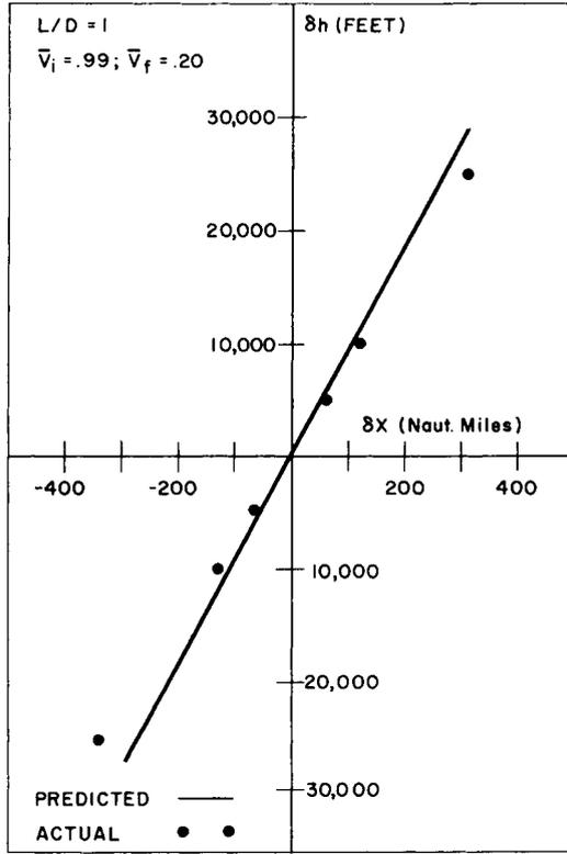
Fig. 5 Comparison between predicted and actual range deviation due to nonequilibrium glide initial condition in altitude
