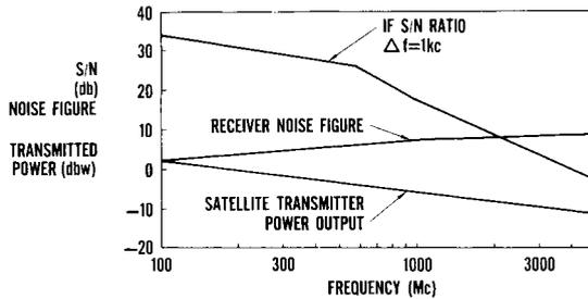
Fig. 3 Signal to noise ratio in 1 kc bandwidth for assumed power and noise figure
