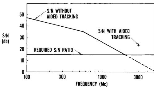
Fig. 5 Output signal to noise ratio
