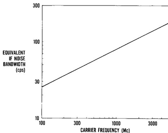
Fig. 4 Bandwidth required to pass doppler data
