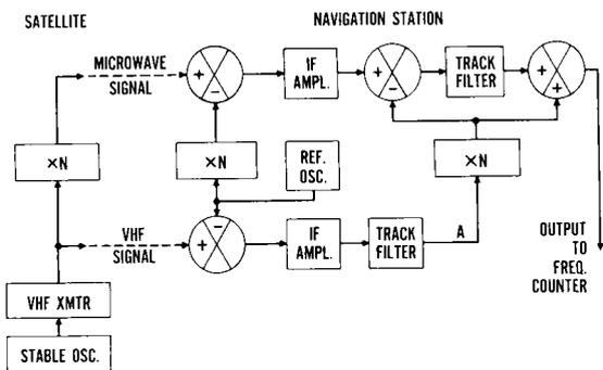
Fig. 7 Proposed passive Doppler system
