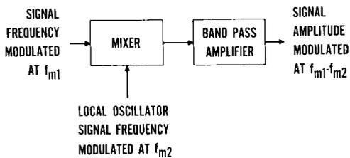
Fig. 9 Sideband folding technique
