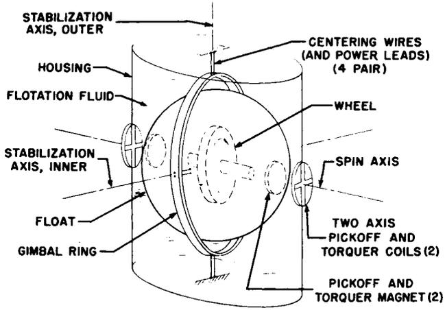
Fig. 1 Functional construction of G8 and  $10^7$  gyros
