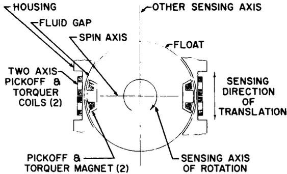
Fig. 2 Pickoff and torquer construction
