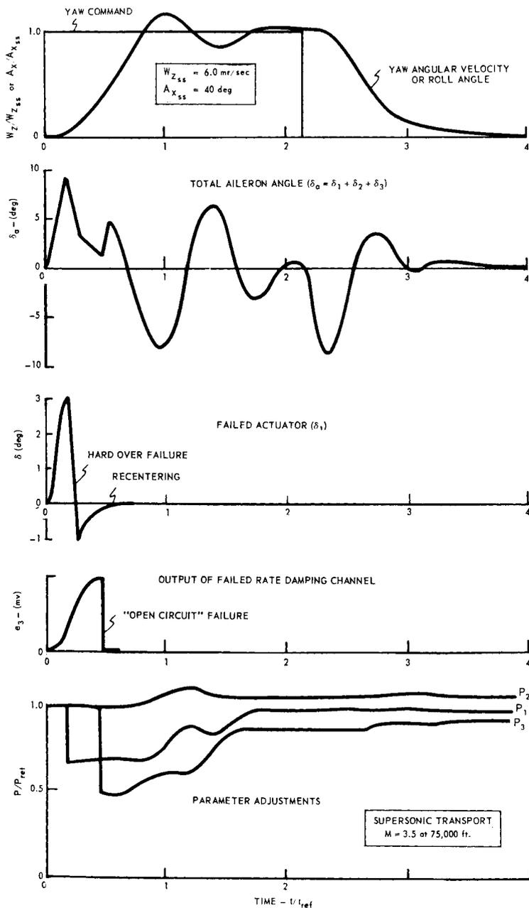
Fig. 7a Operation of the adaptive yaw orientation control system in the event of a compound failure during the response to an input command; adaptive system operating
