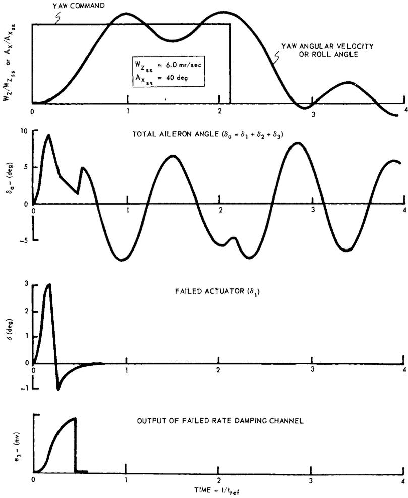
Fig. 7b Response of the yaw orientation control system in the event of a compound failure during the response to an input command; no adaptation
