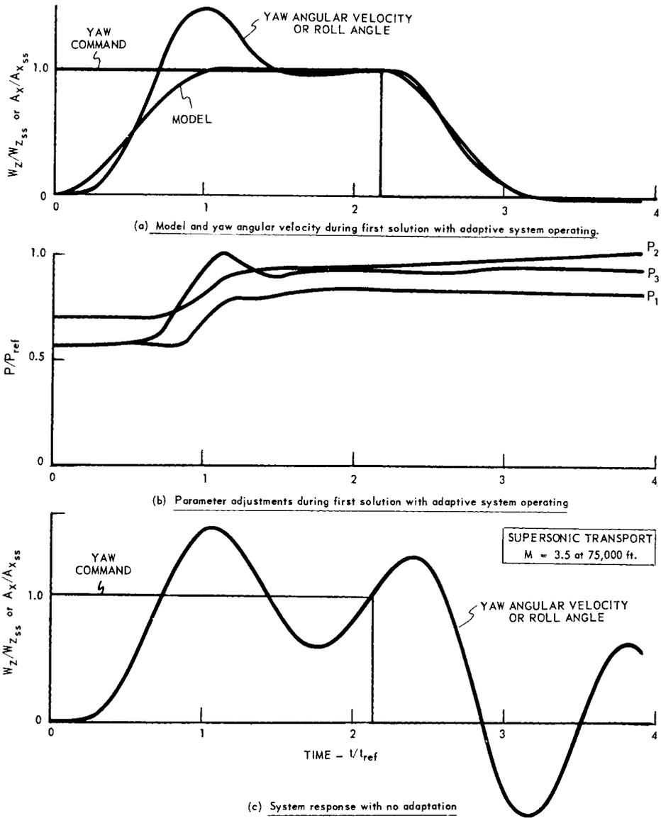
Fig. 5 Typical operation of the adaptive yaw orientation control system with the loop gains offset from optimum
