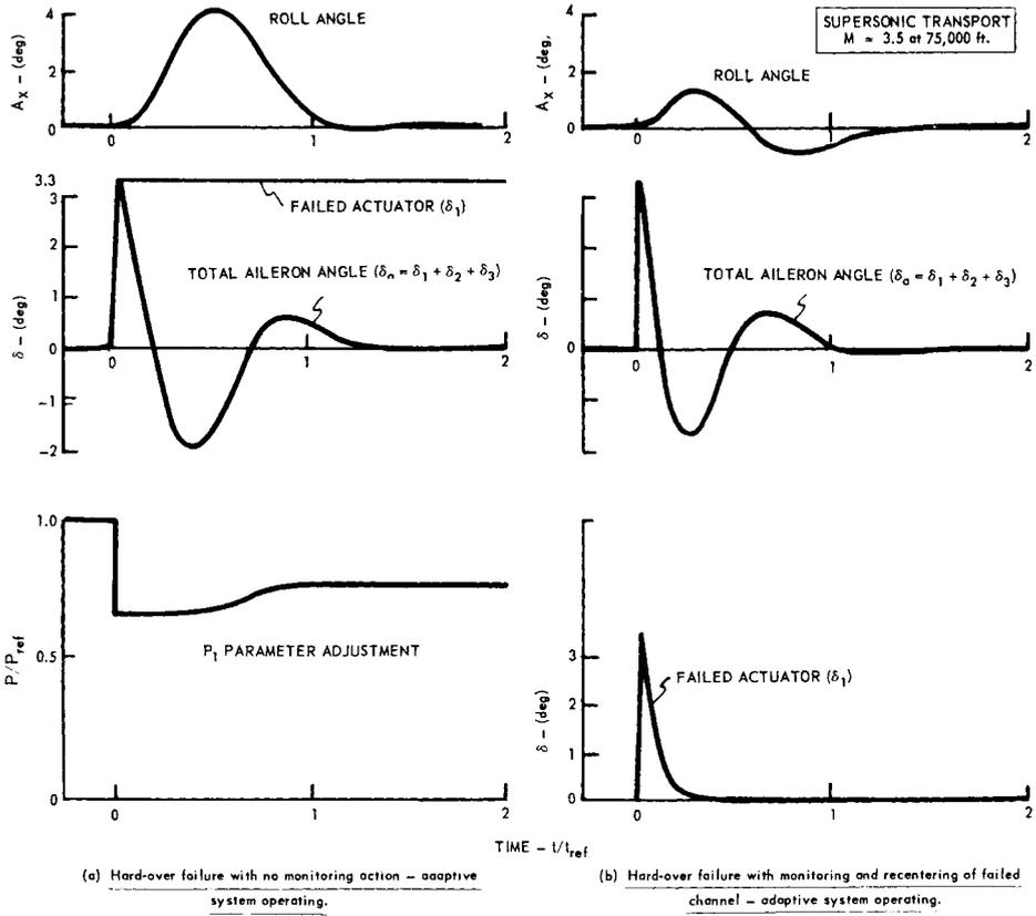
Fig. 6 Operation of the adaptive yaw orientation system in the event of a hard over failure and no input command
