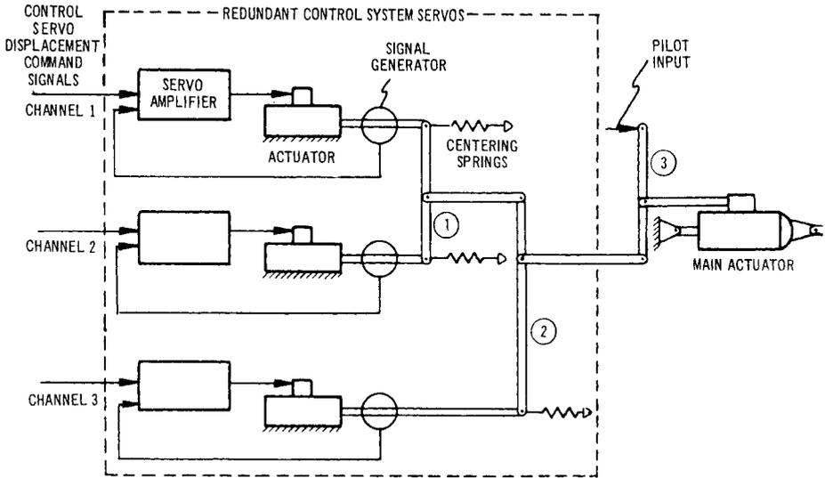
Fig. 4 Schematic diagram of three redundant servos whose output displacements are added mechanically
