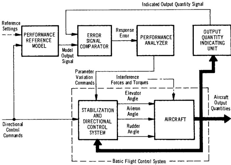
Fig. 1 Simplified functional diagram for a model reference adaptive flight control system
