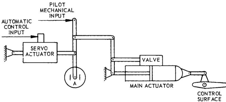
FOR PARALLEL OPERATION: POINT A IS A FIXED PIVOT FOR ROTATION.
