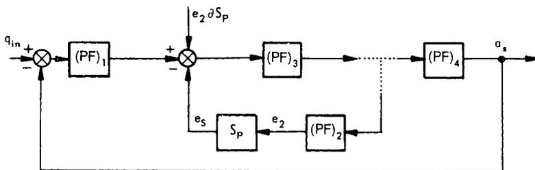
Fig. 9 Generalized control system block diagram
