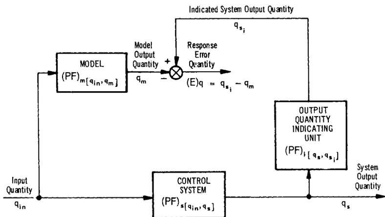
Fig. 8 Mathematical block diagram representation of a model reference adaptive control system
