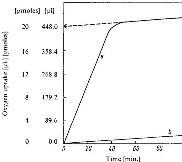
Fig. 1. Time course of the manometric determination of 40  $\mu\text{moles}$  D-lactate in the presence of 40  $\mu\text{moles}$  L-lactate (Curve a). Curve b: Oxygen uptake with 40  $\mu\text{moles}$  L-lactate.
