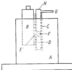
Fig. 5. A simple housing for photomultiplier and sample
