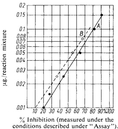
Fig. 3. Standard curves for (A) diethyl-*p*-nitrophenyl phosphate (Paraoxon) and (B) *O,O*-diethyl-*O-p*-nitrophenyl thiophosphate (Parathion). The latter after oxidation with a mixture of equal volumes of conc. and fuming  $\text{HNO}_3^*$ .
