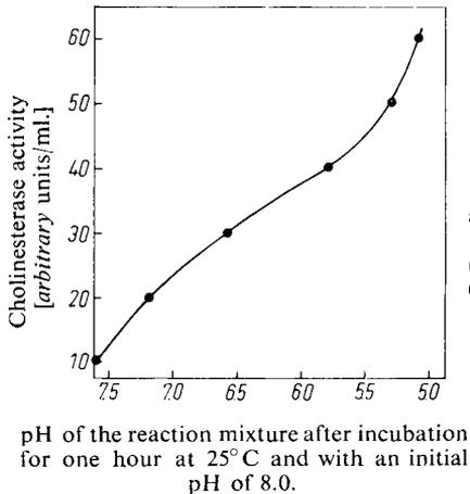
Fig. 2. Standard curve for the hydrolysis of acetylcholine by cholinesterase (1 hour at  $25^\circ\text{C}$ ). Reaction mixture: 3 ml. buffer (solution I); 3 ml. cholinesterase solution; 0.6 ml. acetylcholine standard solution (V)
