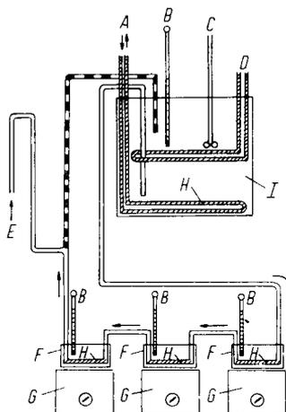
Fig. 1. Diagram of the constant temperature apparatus: A = cooling water; B = thermometer; C = stirrer; D = heating element with thermostat; E = tube for compressed air; F = small, insulated constant temperature baths (crystallization dishes); G = magnetic stirrers; H = copper coil; I = large constant temperature water bath.
