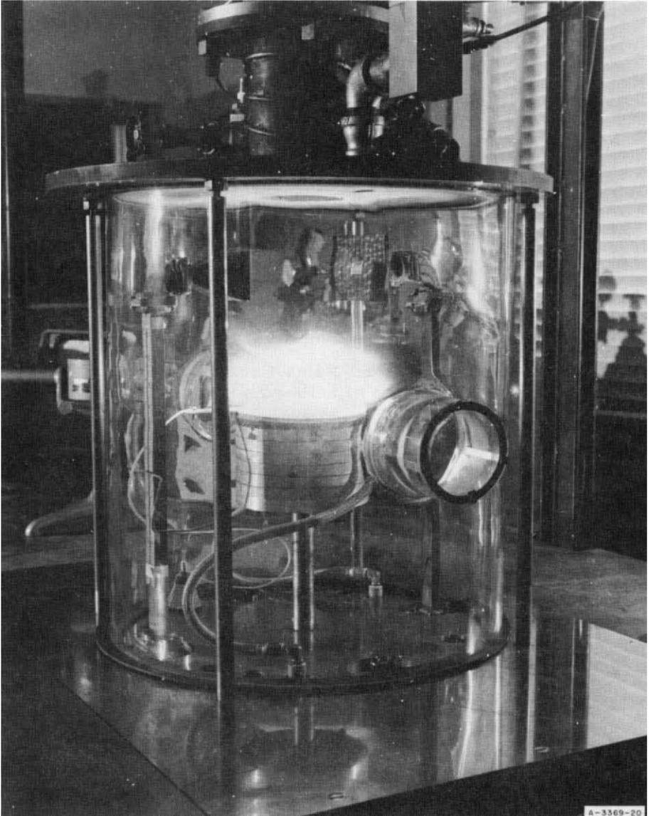
Fig. 5. Ethylene-Oxygen Flame Burning at 8 mm Hg Pressure.
