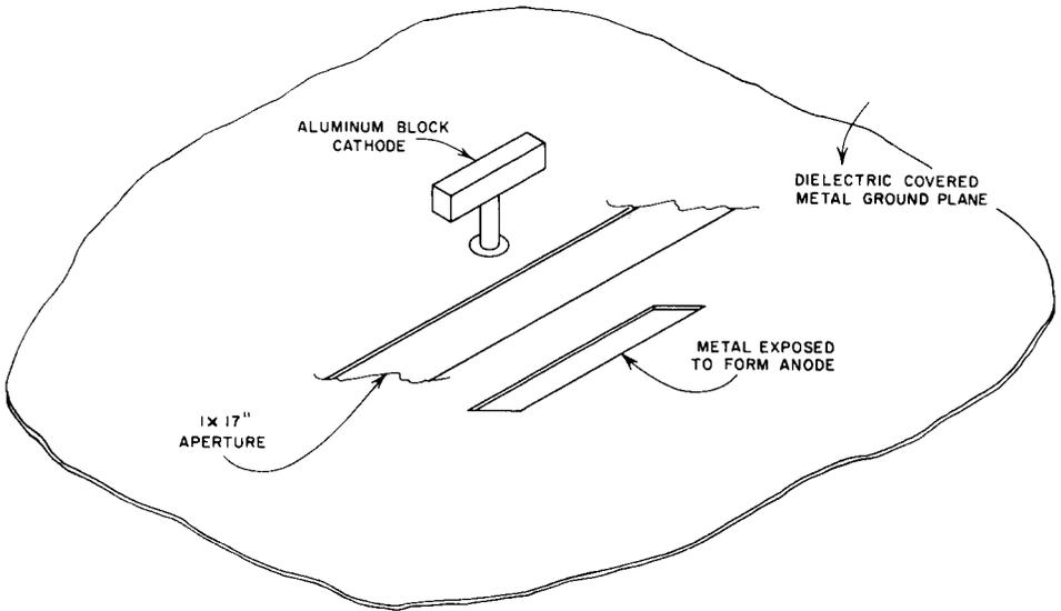
Fig. 1. Configuration Used in Producing a DC Plasma Over Surface of Slot Antenna.
