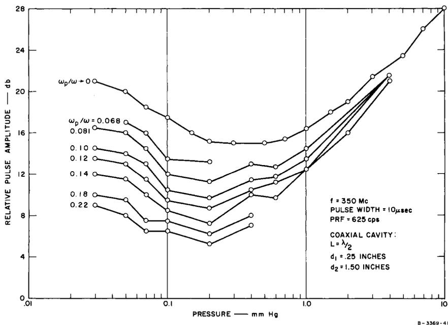
Fig. 3. Effect of a Plasma, Occurring in the Afterglow of an RF Discharge, on the Breakdown of Air in a Coaxial Cavity.
