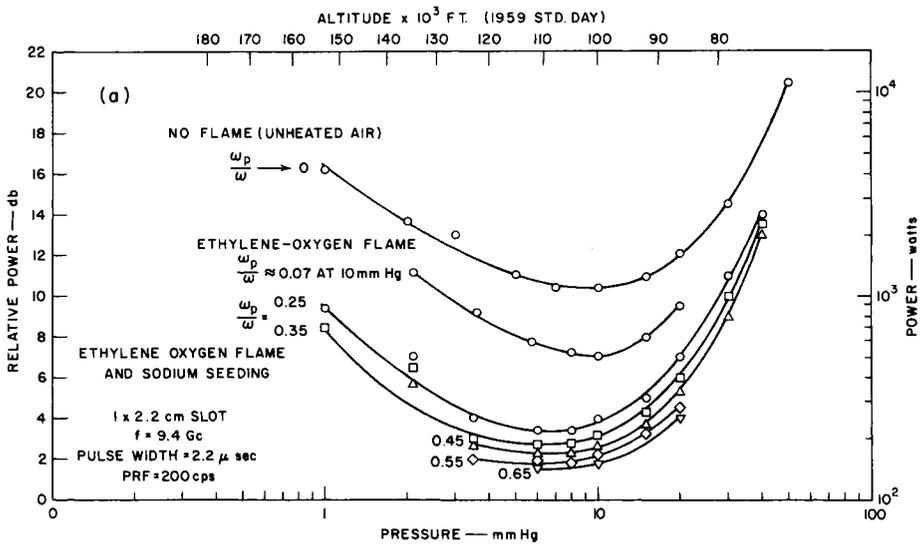
Fig. 6. Measured X-Band Pulse Breakdown Power Levels in the Presence of a Plasma.
