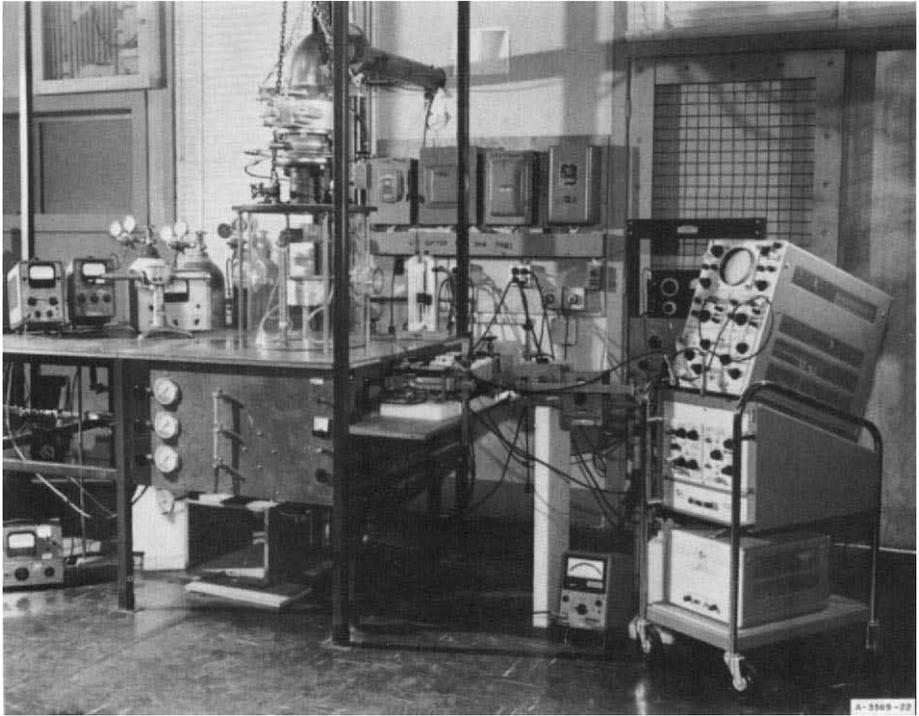
Fig. 4. Low Pressure Flame Experimental Set-up.
