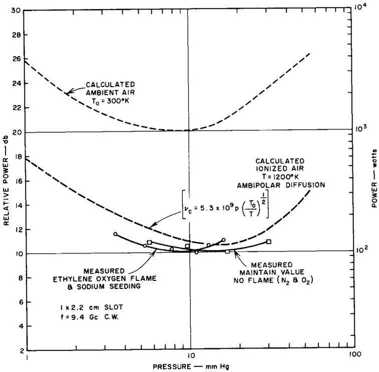
Fig. 9. Measured and Calculated X-Band CW Breakdown Power Levels in the Presence of a Plasma.
