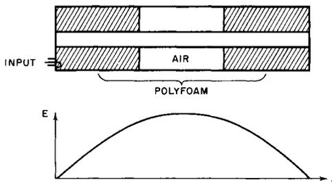
Fig. 2. Drawing of Coaxial Cavity Used in Afterglow Experiments and the Fundamental-Mode Electric Field Distribution Along the Length of the Cavity.
