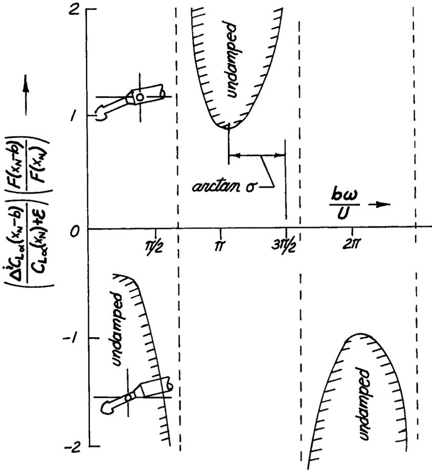
Fig. 5. (a) Stability Boundary of an Arbitrary Bending Mode Throughout Speed Range,  $b\omega/U$ , for a Specific Vehicle.
