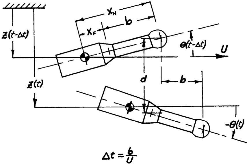
Fig. 4. Position of Vehicle at Two Instants of Time
