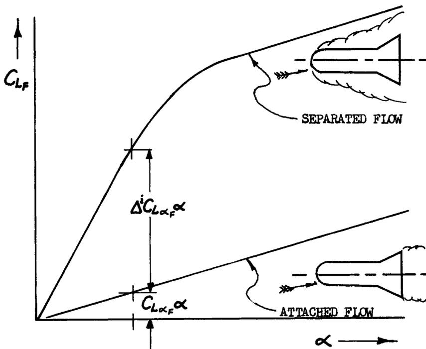
Fig. 2. Flare Lift of a Blunt Body of Revolution.
