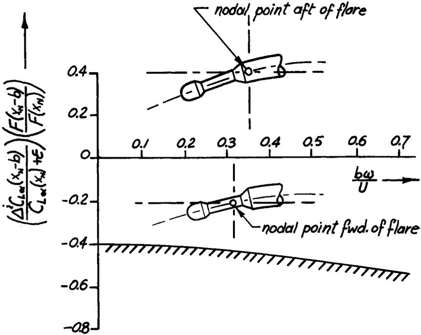
Fig. 6. Stability Boundary of an Arbitrary Bending Mode for a Specific Vehicle at Low Reduced Frequency.
