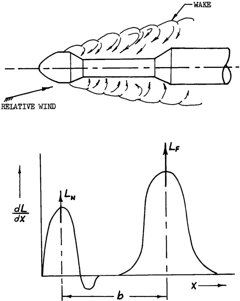
Fig. 1. Force Distribution in Wake of Separated Flow.
