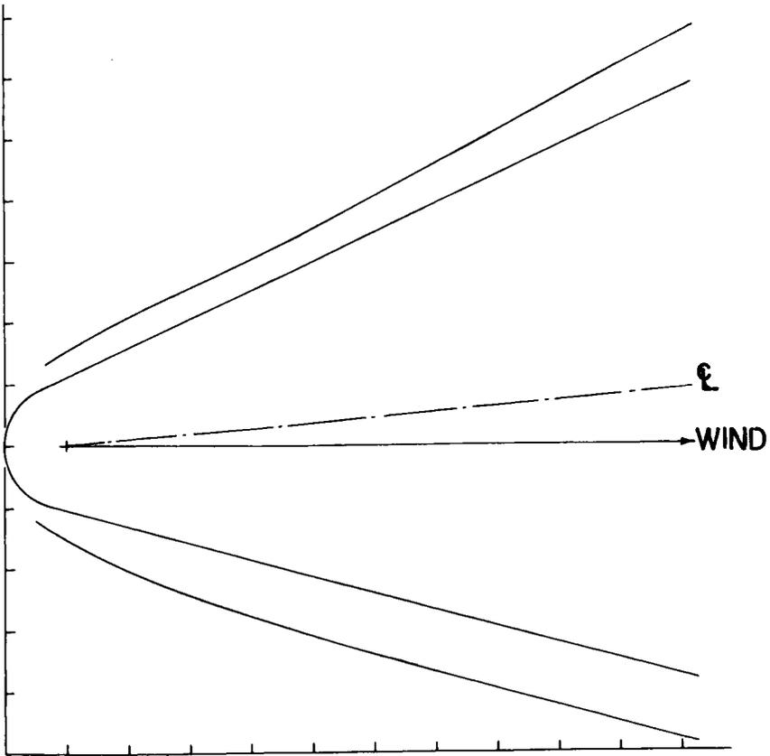
Fig. 9. Side View of a Blunted Yawed Cone and Its Shock Wave at  $M = 8$ .
