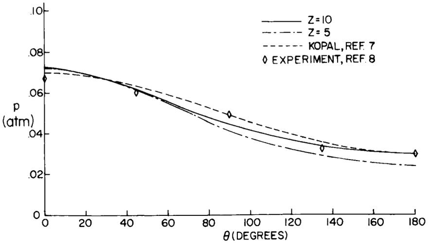
Fig. 11. Cross-Distribution of Pressure on a Yawed Cone.
