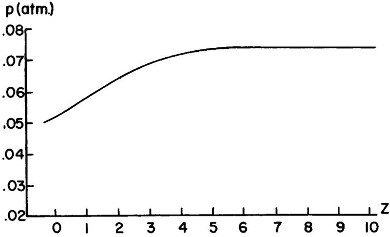
Fig. 10. Axial Pressure Distribution on the Windward Side of a Yawed Cone
