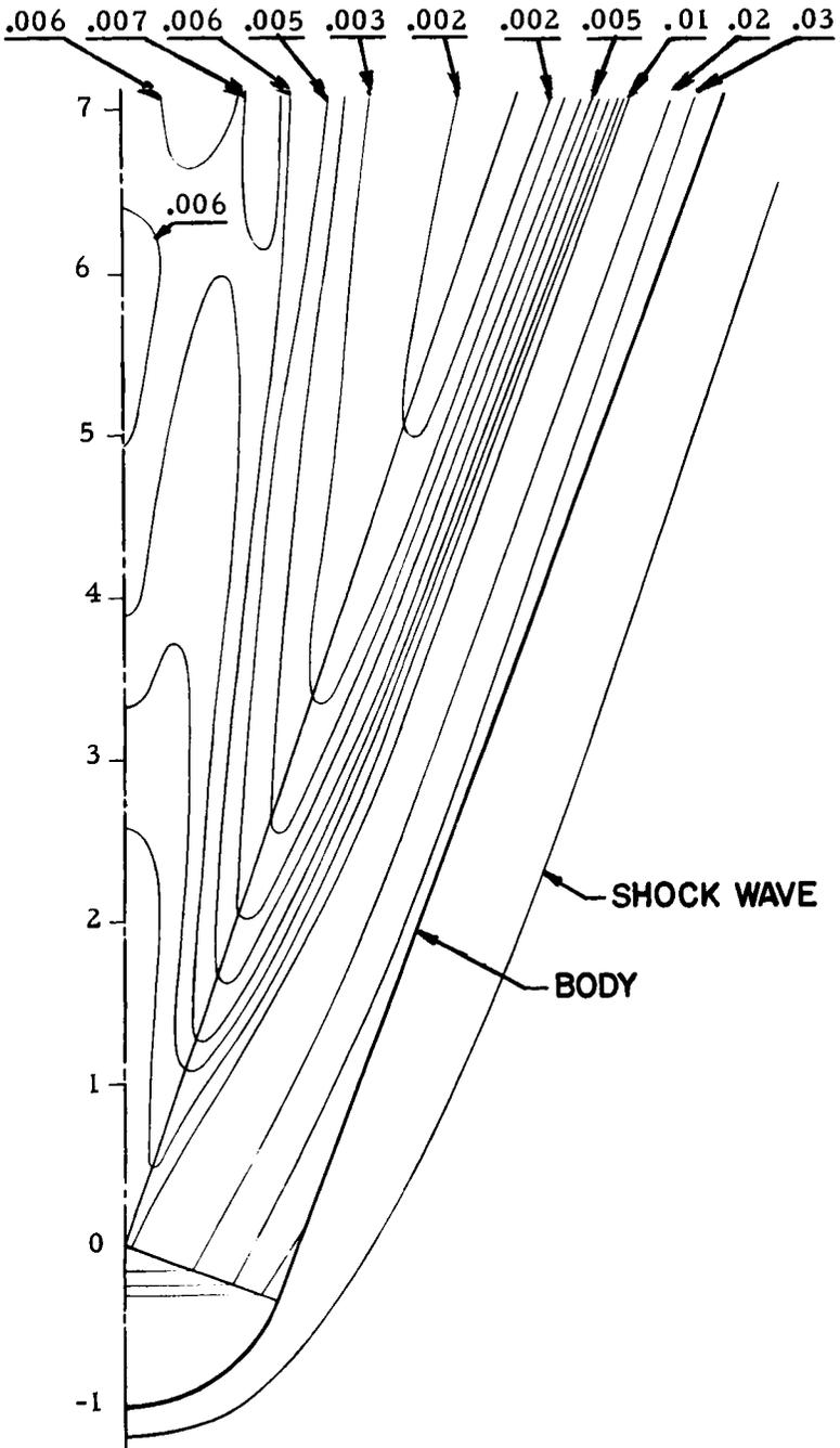
Fig. 8. Pressure Distribution on a Delta Wing (Atm).
