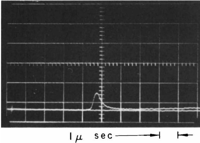
Fig. 12 Oscilloscope of the nitrogen first positive radiation behind a normal shock in air in the electric shock tube. The wavelength region is 5000A - 10,000A,  $U_s = 33,000$  fps,  $P_1 = 0.1$  mm Hg.
