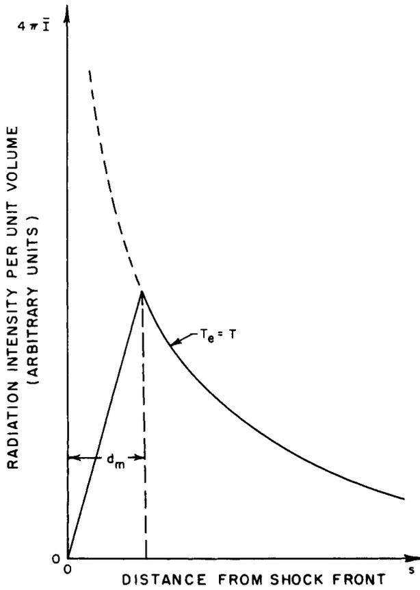
Fig. 5 Schematic diagram of radiation profile. For  $s \geq d_m$ , it is assumed that  $T_e = T$ . For  $s < d_m$ ,  $\bar{I}$  increases linearly with  $s$ .
