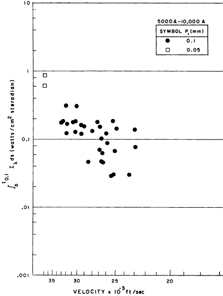
Fig. 15 Integrated luminous front intensity for the  $N_2(1+)$  band system in air as a function of the reciprocal of the shock speed. The integration is carried out to a distance behind the shock front at which the radiation intensity is 10% higher than the equilibrium level.
