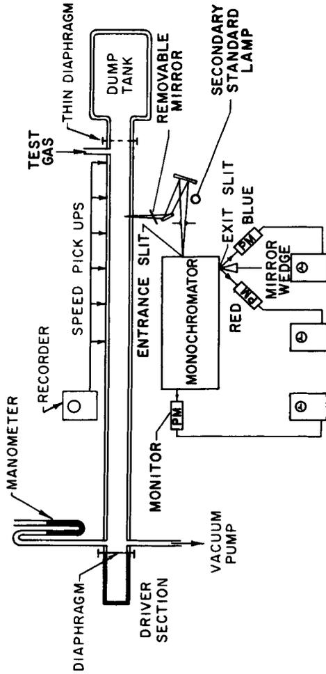
Fig. 8 Schematic diagram of 1.5 in. combustion-driven shock tube. The removable mirror and secondary standard lamp are used in the calibration procedure.
