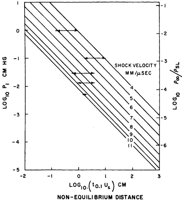
Fig. 17 Initial pressure  $P_1$  is plotted against luminous front thickness  $d_{0.1}$  for various shock speeds. In the laboratory coordinate system  $d_{0.1} = U_s t_{0.1}$ . The lines have been constructed by means of the empirical curve of Fig. 16. Arrows indicate the regions covered by the experiment.
