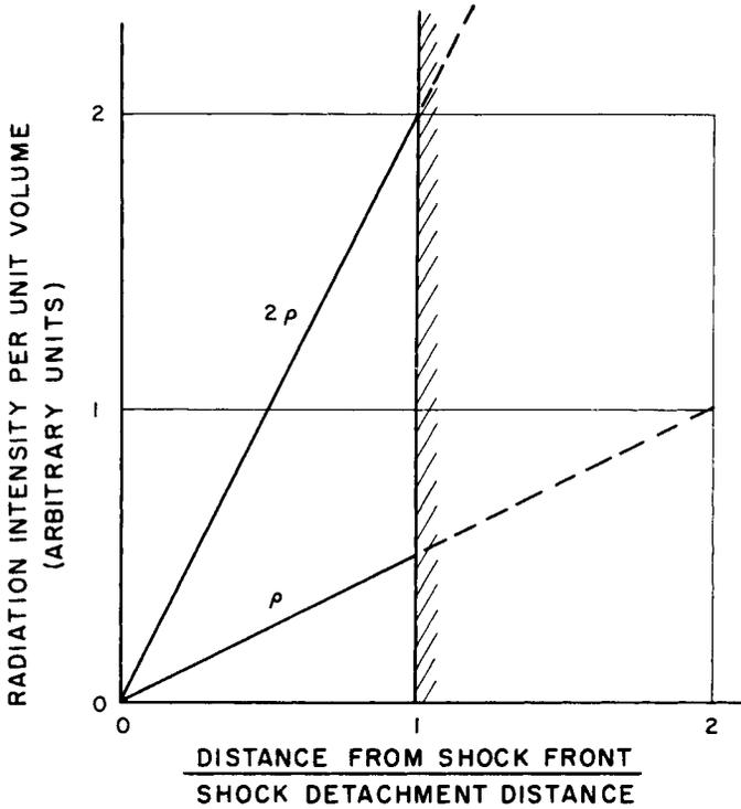
Fig. 3 Schematic diagram of luminous front truncation for a linear rise of radiation intensity. A factor of 2 increase in ambient density results in a fourfold increase in radiation intensity at a given distance behind the shock front, leading to a  $\rho^2$  dependence for the integrated intensity behind a truncated shock front.
