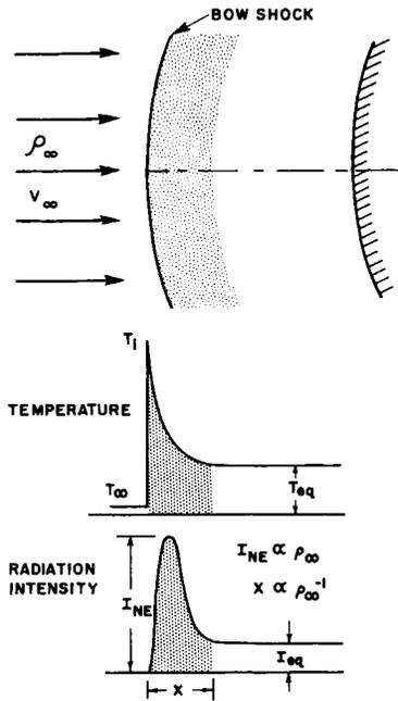
Fig. 1 Schematic diagram of the nonequilibrium region behind the bow shock at the stagnation point of a blunt body.
