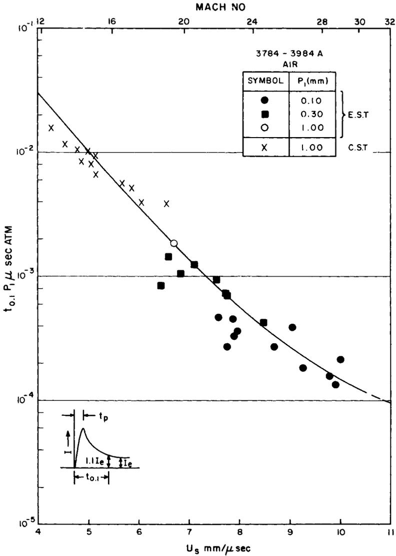
Fig. 16 Observed time duration of luminous front in air, plotted versus shock speed. The time  $t_{0.1}$  in the laboratory coordinate system is taken to a point at which the radiation intensity has decayed to a level 10% above equilibrium. Initial pressure is used as a scaling factor to correlate data obtained at different values of  $P_1$ . The solid line is an empirical curve drawn through the data.
