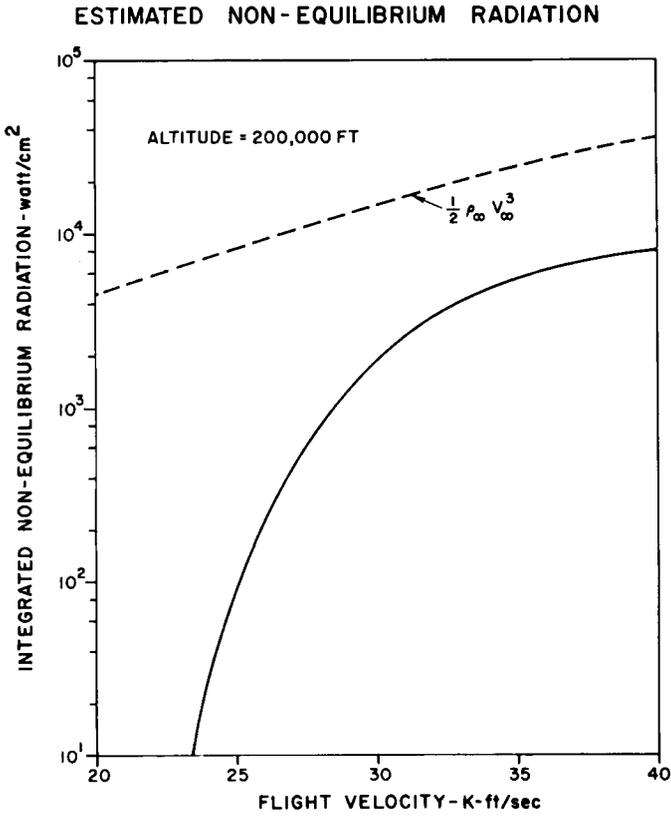
Fig. 6 Preliminary estimate of the integrated nonequilibrium radiation as a function of flight velocity at 200,000 ft altitude. The solid curve shows the results of calculations based on a very tentative model of the relaxation region. It is presented purely to stress the need for experimental measurements in this velocity range. The broken curve shows the incident energy flux per unit area of bow shock.
