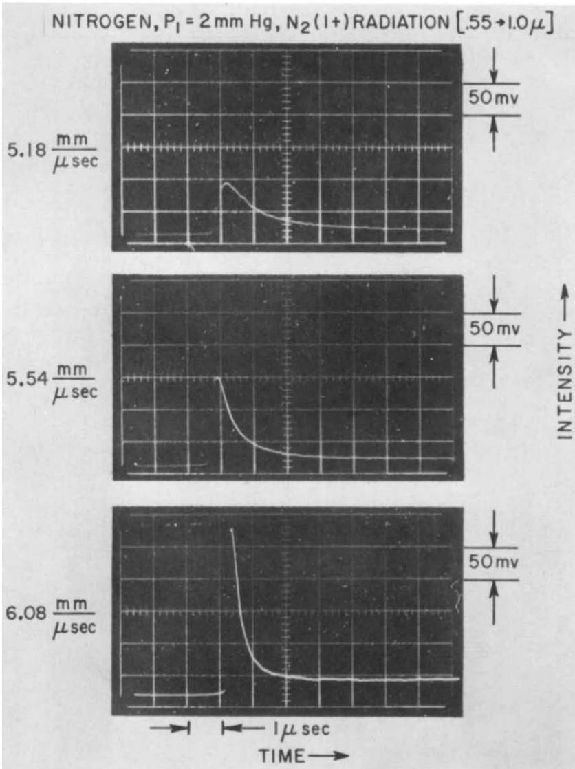
Fig. 9 Typical oscillograms of the nitrogen first positive band system radiation from shock waves in pure  $N_2$  showing the radiation overshoot behind the shock front and subsequent relaxation to equilibrium for several shock speeds.
