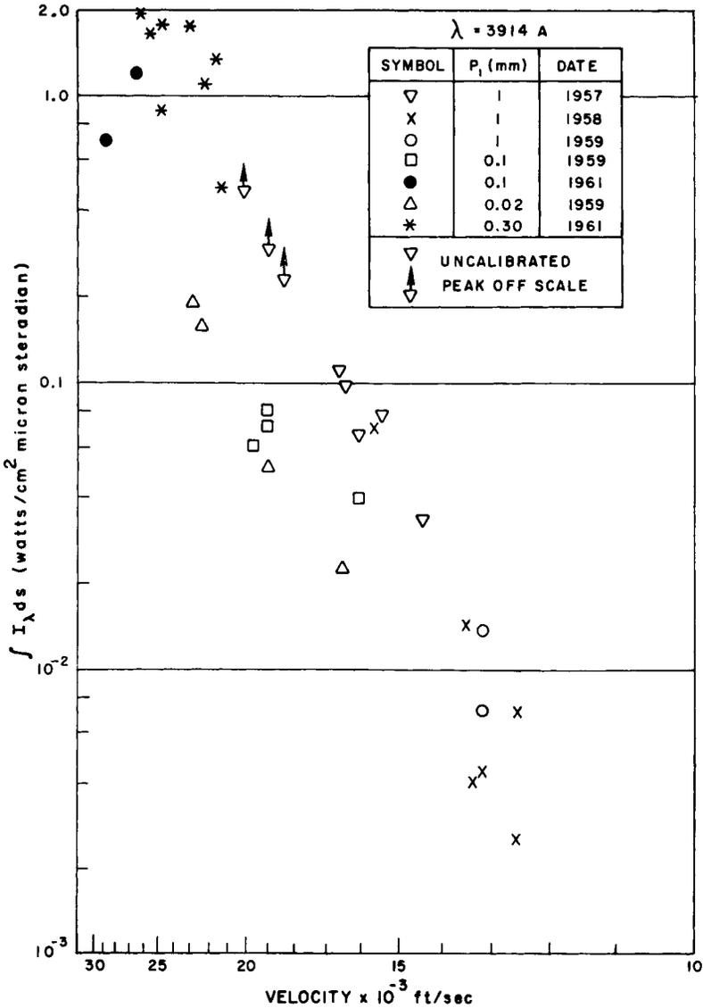
Fig. 14 Integrated luminous front intensity for  $\lambda = 3914\text{\AA}$  in air as a function of the reciprocal of the shock speed. This radiation is due to the  $N_2^+(1-)$  band system. The measurements cover a bandwidth of 200 $\text{\AA}$ . Note that the units of the ordinate scale differ from those of Fig. 15.
