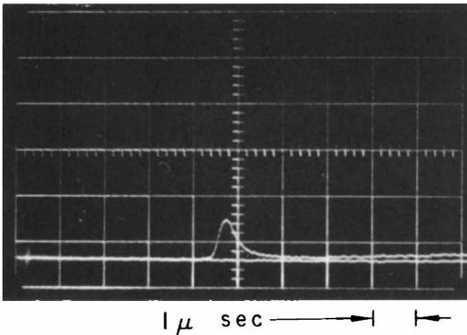
Fig. 13 Time resolved drum camera photograph of normal shock in air in electric shock tube, showing luminous front radiation at left, followed by equilibrium region and driver gas.  $U_s = 33,000$  fps,  $P_1 = 0.1$  mm Hg. The photograph shows the full width of the shock tube, but is distorted in the axial direction. The test slug is approximately 7 cm in length.
