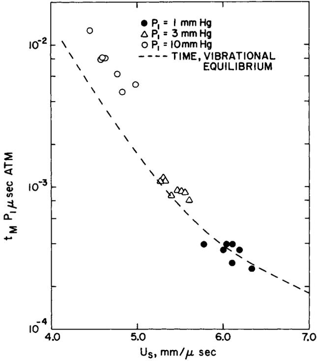
Fig. 18 Observed time of peak radiation  $t_M$  for the  $N_2(1+)$  system in pure nitrogen, plotted vs. shock speed. Initial pressure is used as a scaling factor to correlate data obtained at different values of  $P_1$ . The calculated time for equilibration of the vibrational degrees of freedom of the molecules is also shown.
