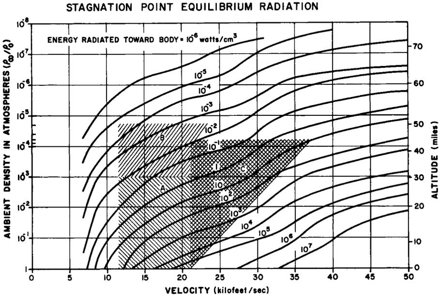
Fig. 10 Approximate operating regions for shock tube radiation measurements in terms of shock velocity and ambient air density.
