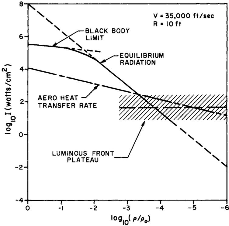
Fig. 19 Comparison of radiative and aerodynamic heat transfer as a function of ambient density for a flight speed of 35,000 fps and nose radius  $R=10$  ft. The location of the luminous front plateau is not yet known. The lower limit shown is based on the measurements of Figs. 14 and 15.
