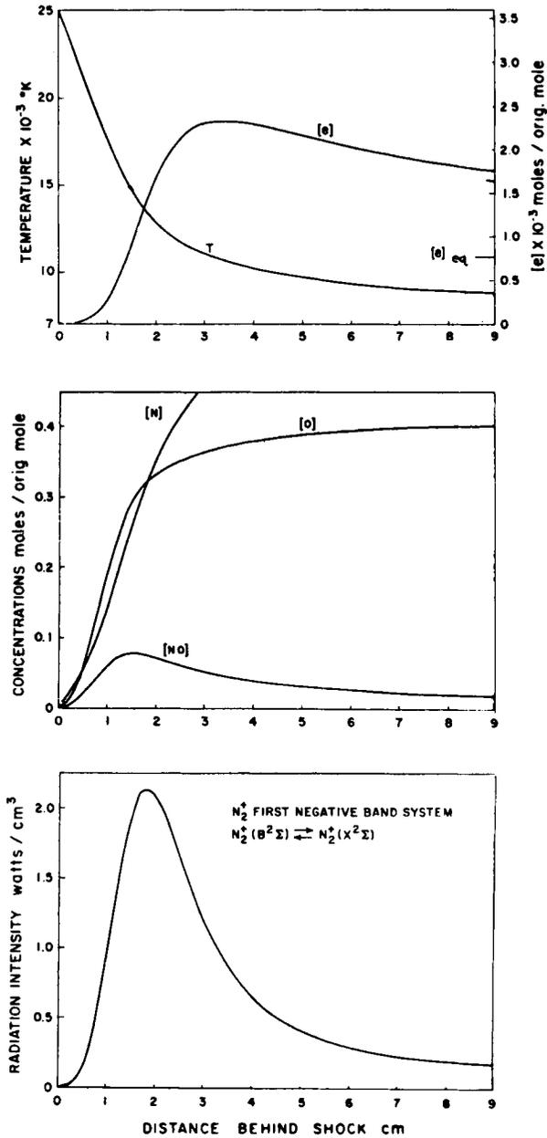
Fig. 4 Relaxation behind a shock wave travelling at 23,500 fps into air at an initial pressure of  $20\mu$  Hg. Concentrations are expressed in moles per mole of unshocked gas. This figure is reproduced from Ref. 5. In view of the revised  $f$  number quoted (Ref. 16) for the  $N_2^+(1-)$  band system, the plotted intensity levels should be reduced by a factor of 2.
