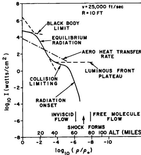
Fig. 2 Comparison of radiative and aerodynamic heat transfer as a function of ambient density for flight speed of 25,000 fps and nose radius  $R = 10$  ft.
