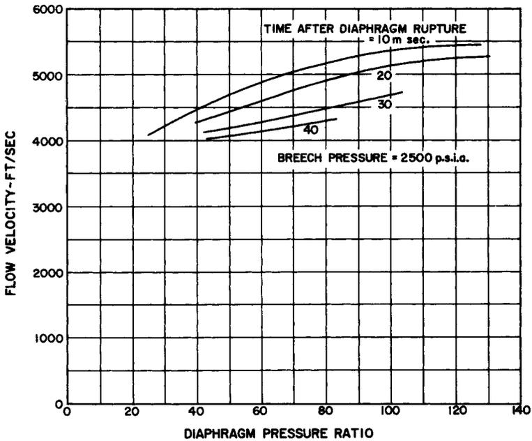
Fig. 17 Flow velocity vs. diaphragm pressure ratio.
