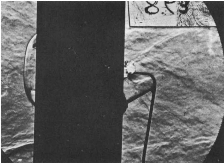
Fig. 26 Schlieren photograph of flow past variable geometry intake (Ref. 22). A strong normal shock wave in front of the intake shows that the internal flow is subsonic.
