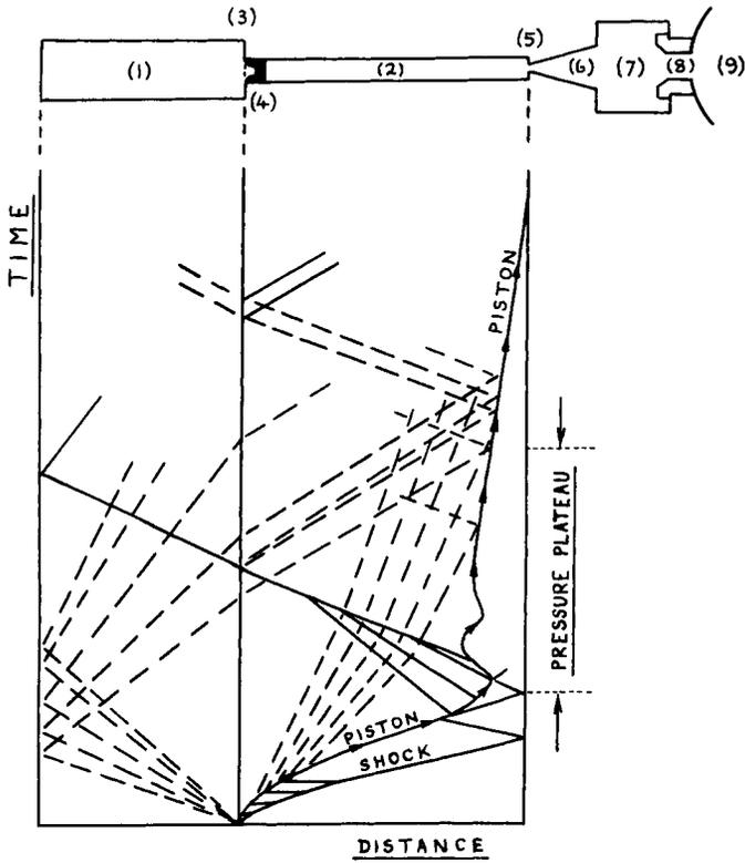
Fig. 1 Gun tunnel and wave diagram.
