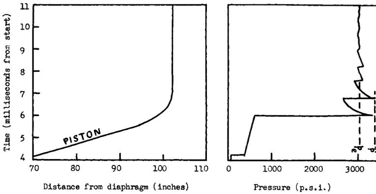
Fig. 14 Portions of  $x-t$  and  $p-t$  diagrams - light piston.  $m_p = 5.5$  gm,  $p_4 = 3015$  psia,  $p_1 = 65$  psia.
