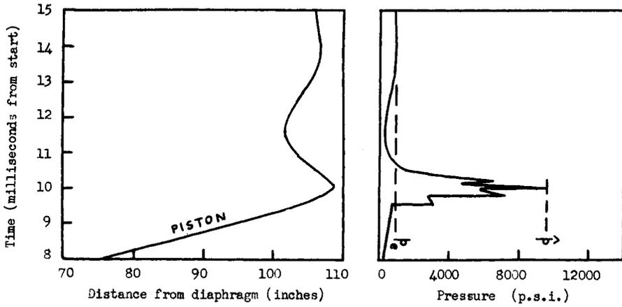
Fig. 12 Portions of  $x-t$  and  $p-t$  diagrams - heavy piston.  $m_p = 15 \text{ gm}$ ,  $p_4 = 975 \text{ psia}$ ,  $p_1 = 15 \text{ psia}$ .
