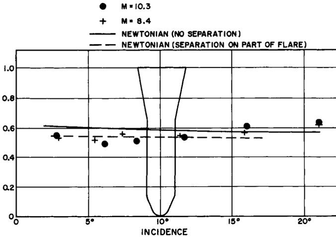
Fig. 23 Center of pressure position vs. incidence for a stand-ard cone-cylinder-flare model: data from 10-in. hyper-sonic gun tunnel at ARDE, Fort Halstead.
