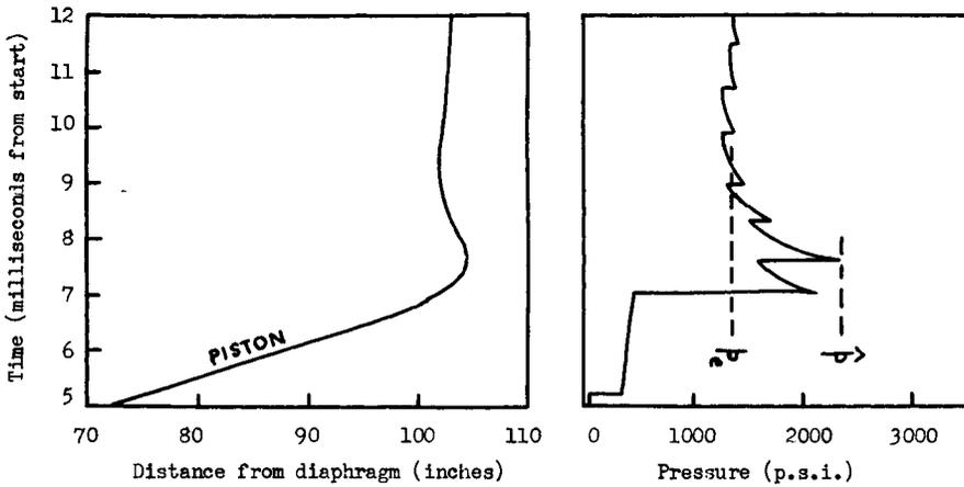
Fig. 13 Portions of  $x-t$  and  $p-t$  diagrams - medium piston.  $m_p = 9 \text{ gm}$ ,  $p_4 = 1275 \text{ psia}$ ,  $p_1 = 40 \text{ psia}$ .
