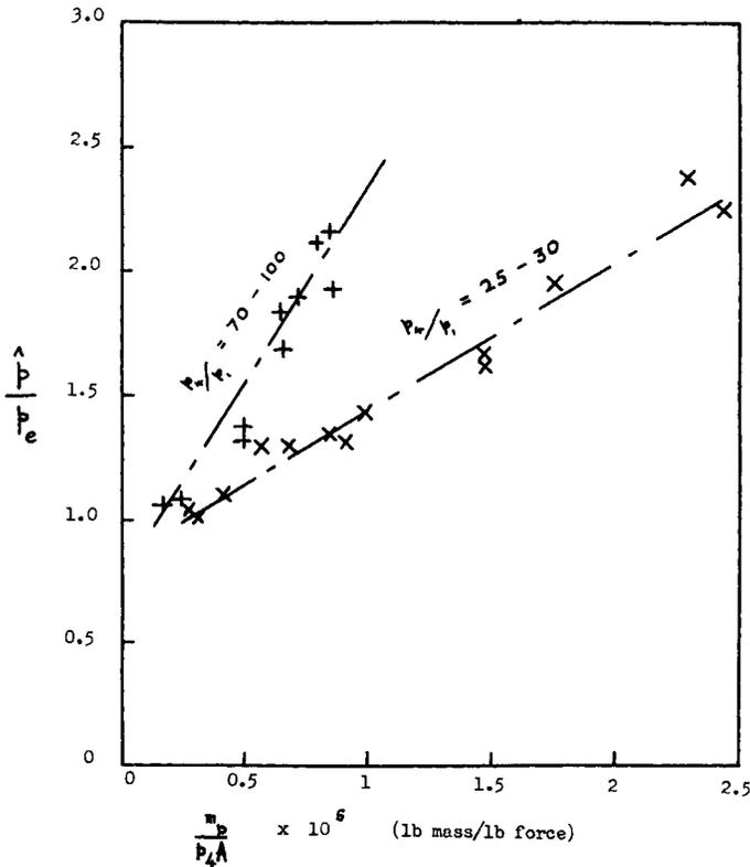
Fig. 15 Ratio of peak pressure to equilibrium pressure plotted against piston mass parameter.
