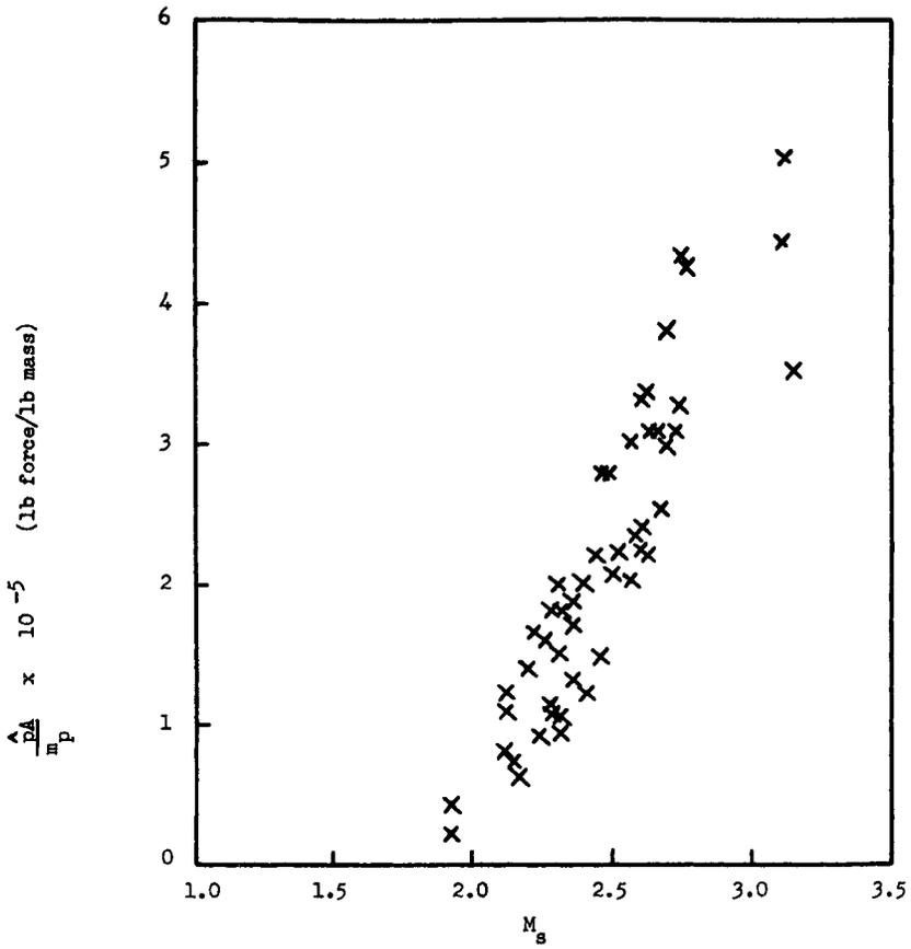
Fig. 8 The variation of a peak pressure parameter with primary shock Mach number.
