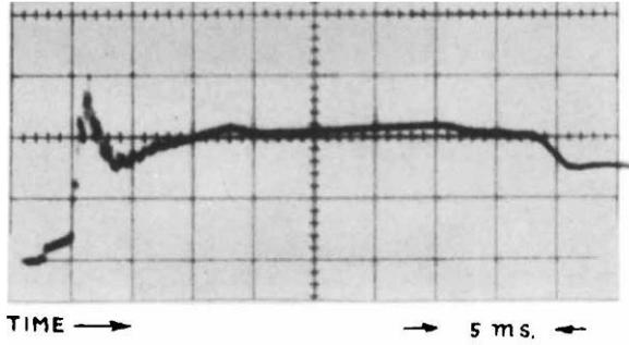
Fig. 5 Pressure - time record at end of low pressure tube - first plateau.  $p_4 = 2160$  psia,  $p_1 = 35$  psia,  $m_p = 8.35$  gm.
