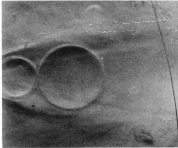
Fig. 16 Typical double - exposure spark schlieren picture of cylindrical disturbance in flow at a Mach number of 11.
