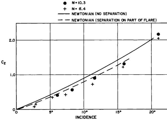
Fig. 22 Normal force coefficient vs. incidence for a standard cone-cylinder-flare model: data from 10-in. hyper-sonic gun tunnel at ARDE, Fort Halstead.
