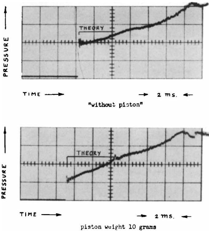
Fig. 3 Pressure - time records at end of low pressure tube - effect of piston on primary shock strength with tube end open.  $p_4 = 360$  psia,  $p_1 = 14.7$  psia.
