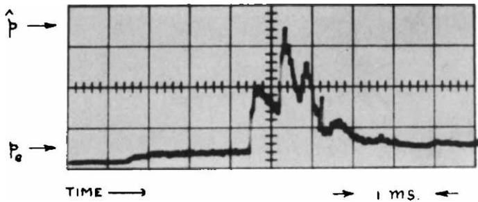
Fig. 4 Pressure - time record at end of low pressure tube - shock reflection process.  $p_4 = 1940$  psia,  $p_1 = 32.7$  psia,  $m_p = 15$  gm.
