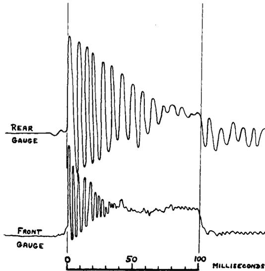
Fig. 21 Typical strain gage balance record for a model in the 10-in, hypersonic gun tunnel at ARDE, Fort Halstead.
