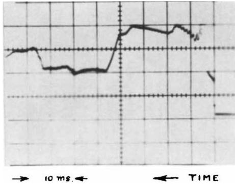
Fig. 6 Pressure - time record at end of low pressure tube - without restrictor plate.  $p_4 = 1055$  psia,  $p_1 = 34.7$  psia,  $m_p = 5.65$  gm.
