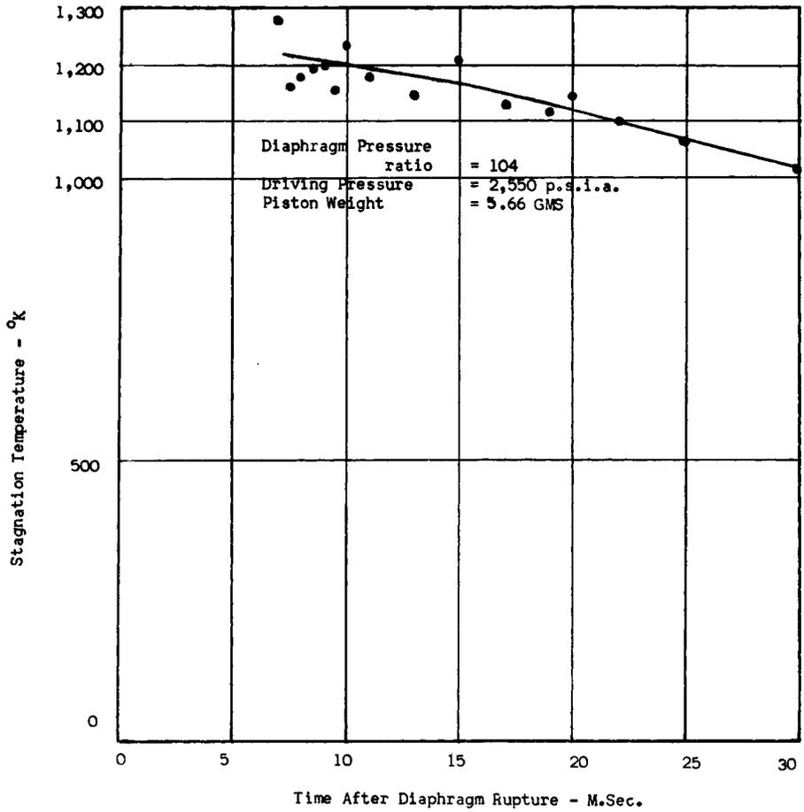
Fig. 19 Stagnation temperature vs. time in run.
