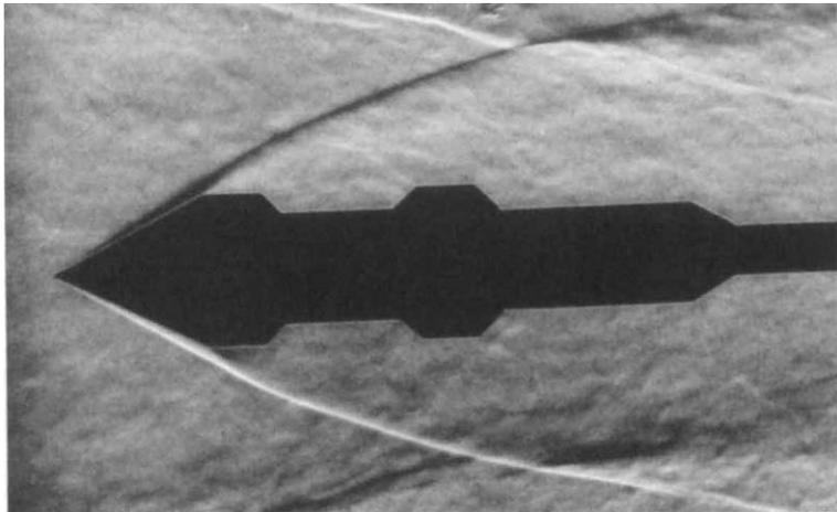
Fig. 11 Spark schlieren photograph of flow past axisymmetric body at a nominal Mach no. of 11. Effect of high pressure (10 mm Hg) in vacuum tank.  $p_4 = 2930$  psia,  $p_1 = 35$  psia.
