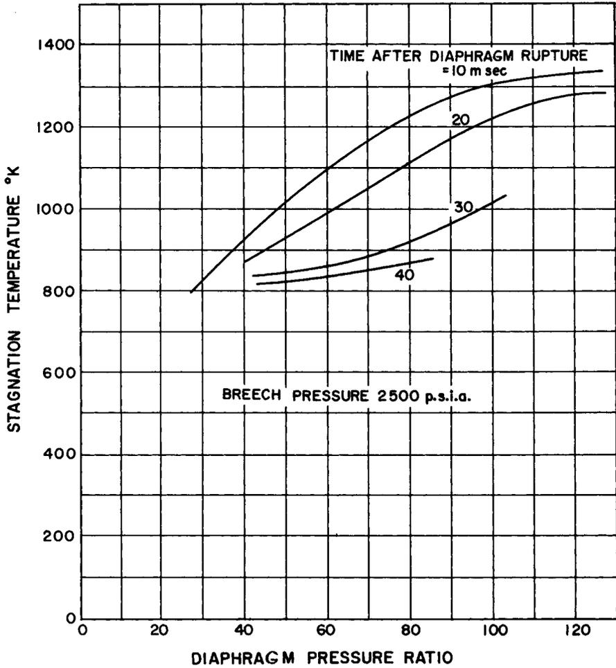
Fig. 18 Stagnation temperature vs. diaphragm pressure ratio.
