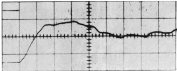
Fig. 9 A typical pitot pressure record on the nozzle center line.  $p_4 = 2700$  psia,  $p_1 = 54.7$  psia, nominal flow Mach number = 11.
