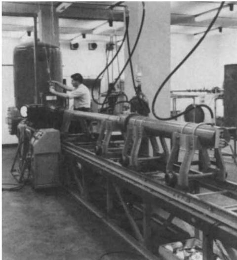
Fig. 2 General view of University of Southampton hypersonic gun tunnel.
