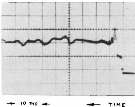
Fig. 7 Pressure - time record at end of low pressure tube - with restrictor plate.  $p_4 = 1045$  psia,  $p_1 = 34.7$  psia,  $m_p = 5.65$  gm.
