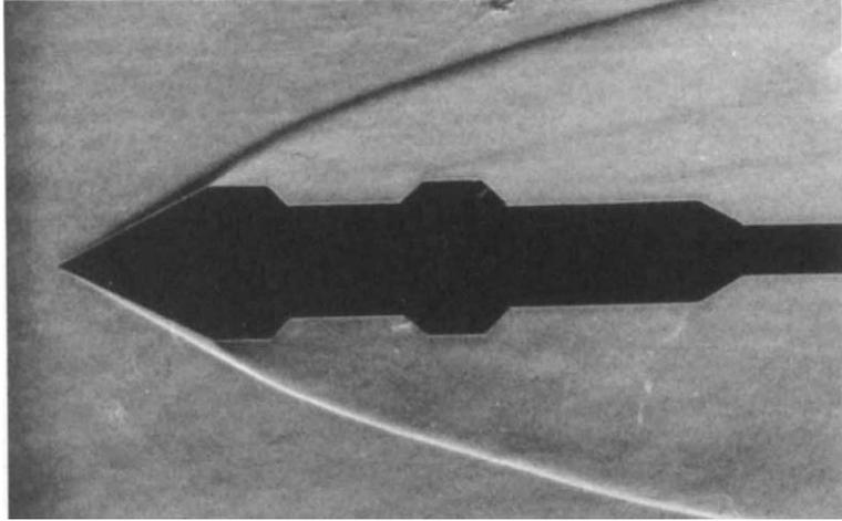
Fig. 10 Typical spark schlieren photograph of flow past axisymmetric body with cut-out to promote separation. Nominal flow Mach number = 11, vacuum tank pressure = 0.1 mm Hg,  $p_4 = 2930$  psia,  $p_1 = 35$  psia.
