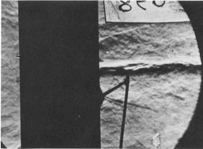
Fig. 25 Schlieren photograph of flow past variable geometry intake (Ref. 22): supersonic internal flow. The position of the movable plates is shown by their leading and trailing edges which project slightly beyond the fixed side plates.
