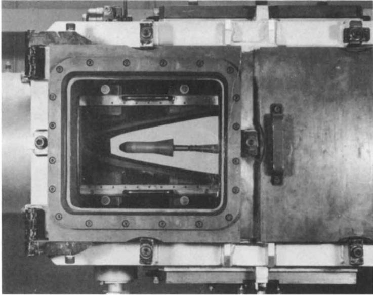
Fig. 20 10-in. diam closed working section of no. 3 hypersonic gun tunnel at ARDE, Fort Halstead.
