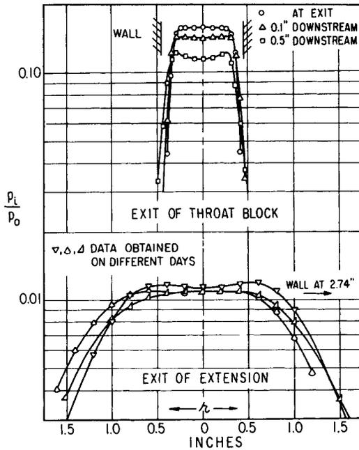
Fig. 4 Radial impact pressure surveys.
