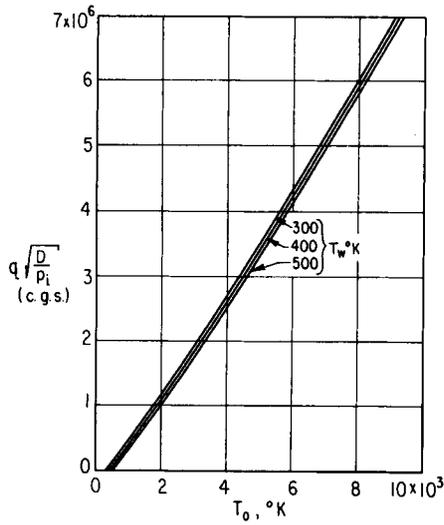
Fig. 7 Stagnation point heat transfer for a flat faced cylinder in Argon;  $M < 4$
