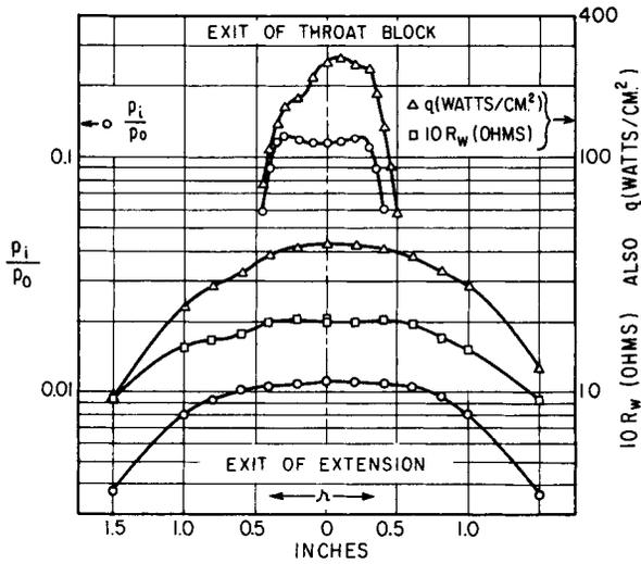
Fig. 8 Comparative heat transfer and impact pressure surveys.
