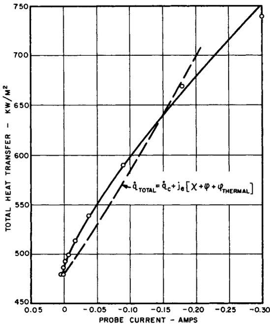
Fig. 12 Conduction plus electron heat transfer for stagnation point probe. ( $j_e$  = electron current density;  $\chi$  = surface work function;  $\phi$  = potential drop across the sheath;  $\phi_{THERMAL}$  = initial thermal energy of the electrons; all in mks units.)
