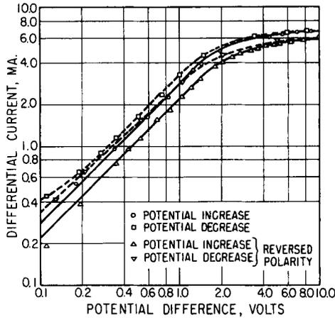
Fig. 13 Stagnation point langmuir probe (configuration B); characteristic curves (0.200 in. off center).
