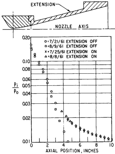
Fig. 3 Axial impact pressure surveys.
