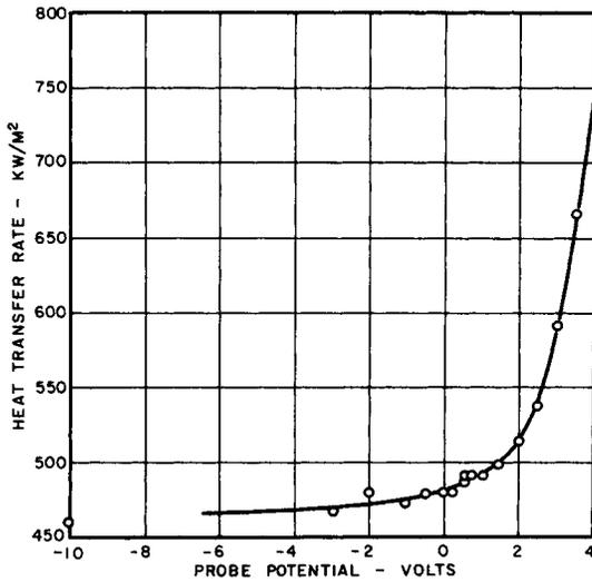
Fig. 11 Effect of prove voltage on stagnation point heat transfer.
