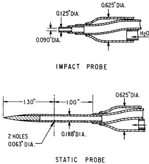
Fig. 2 Water cooled pressure probes.
