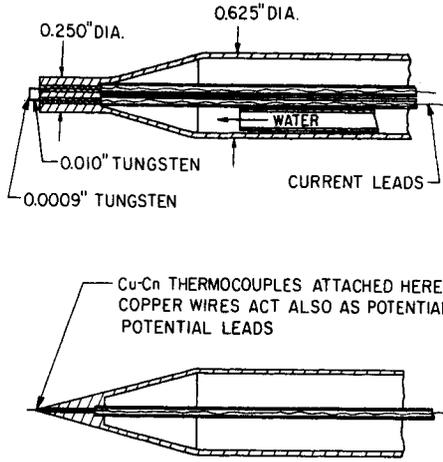
Fig. 9 Free-molecule flow heat transfer probe.
