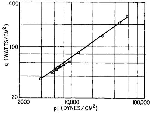
Fig. 10 Heat transfer vs. impact pressure on nozzle axis.
