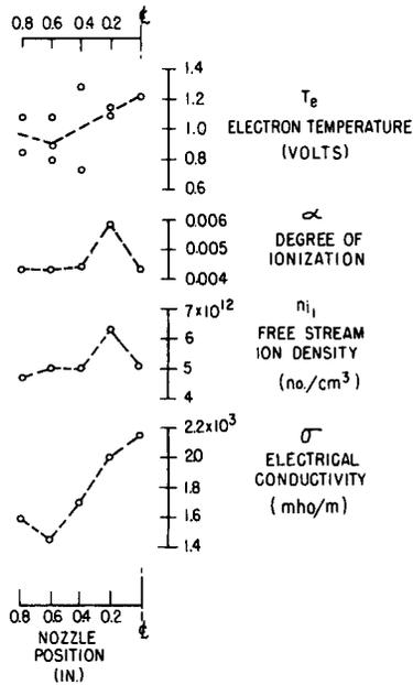
Fig. 14 Electrical properties of stream.
