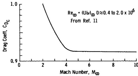
Fig. 15 Drag of spheres at high Reynolds and Mach numbers.
