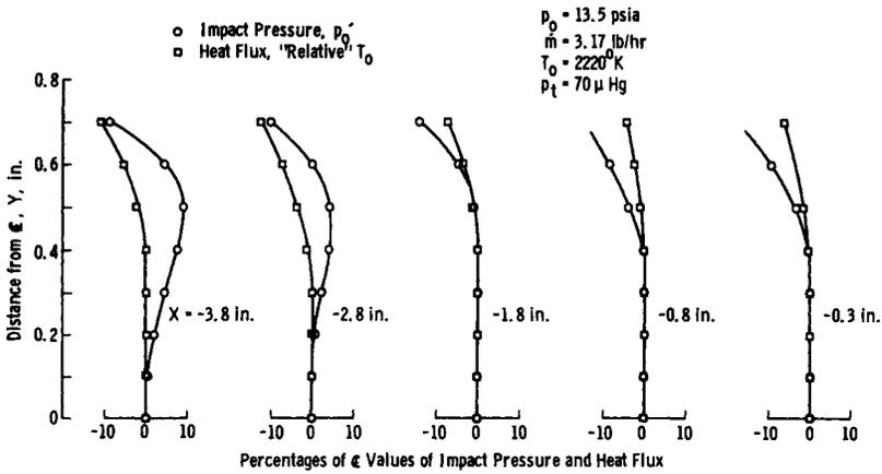
Fig. 9 Typical results of transverse surveys at various axial stations in the LDH tunnel conical nozzle (total angle = 30 deg).
