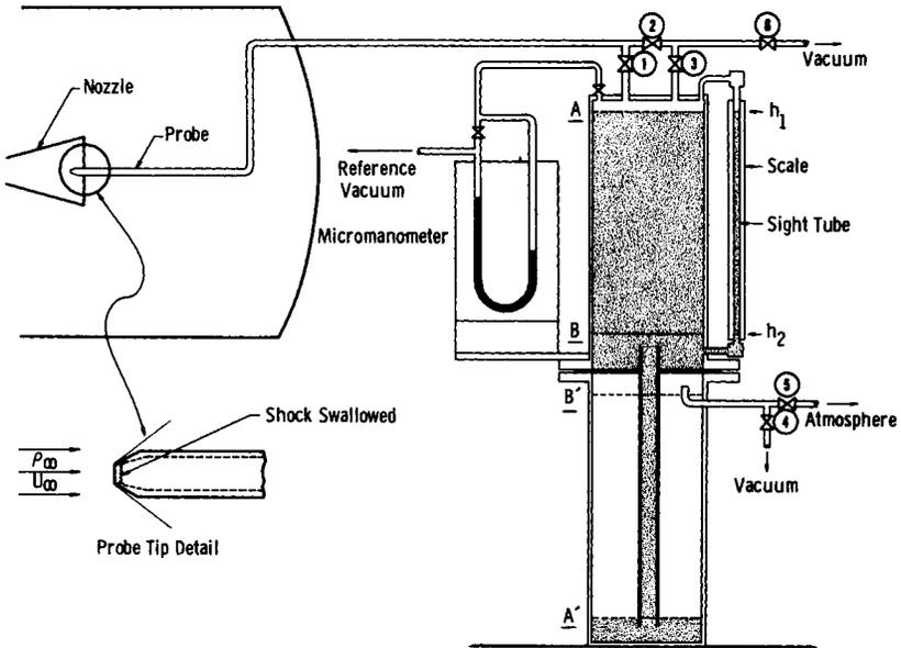
Fig. 7 Diagram of mass flow probe system.
