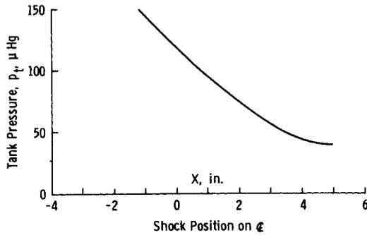
Fig. 14 Effect of tank pressure on shock position.
