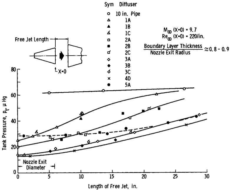
Fig. 12 Diffuser performance with clear jet.
