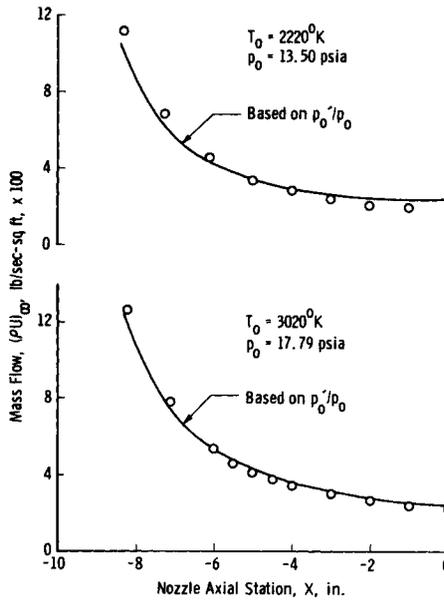
Fig. 8 Measurements with a mass flow probe (points represent local values on nozzle  $\mathcal{E}$  ).
