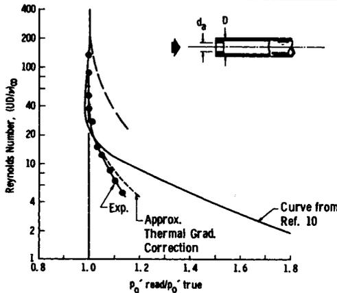
Fig. 5 Viscosity effect on readings of impact pressure probes at low Reynolds numbers and supersonic speeds.
