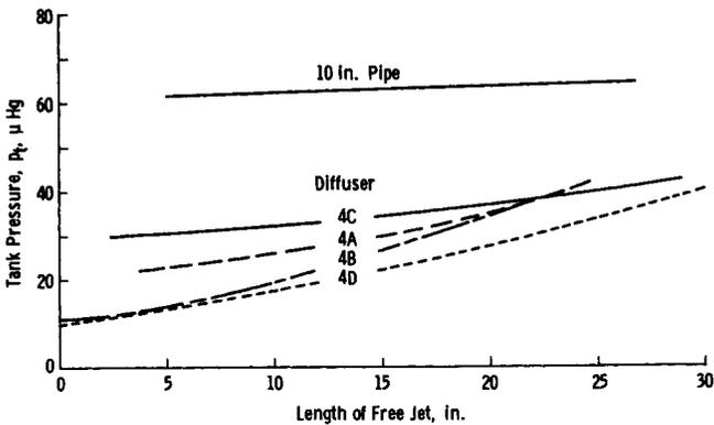
Fig. 13 Diffuser component contributions with clear jet.
