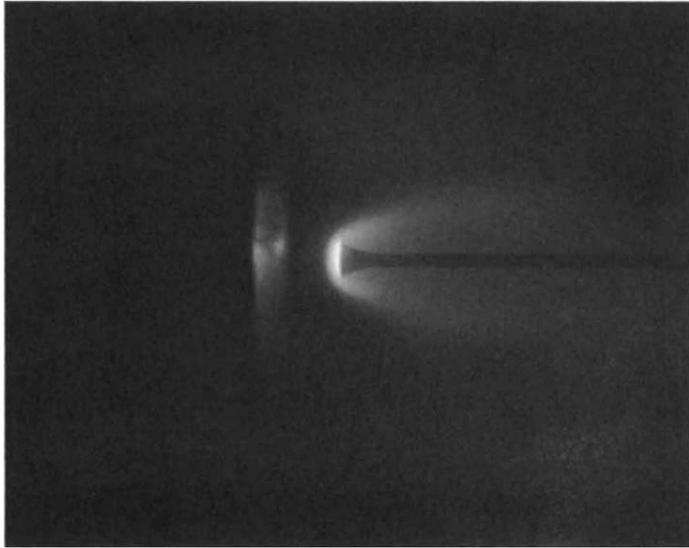
Fig. 4 Flow visualization produced by artificially created electric field;  $M_\infty = 9.7$ ,  $U_\infty = 8700$  fps, equivalent altitude = 50 miles.
