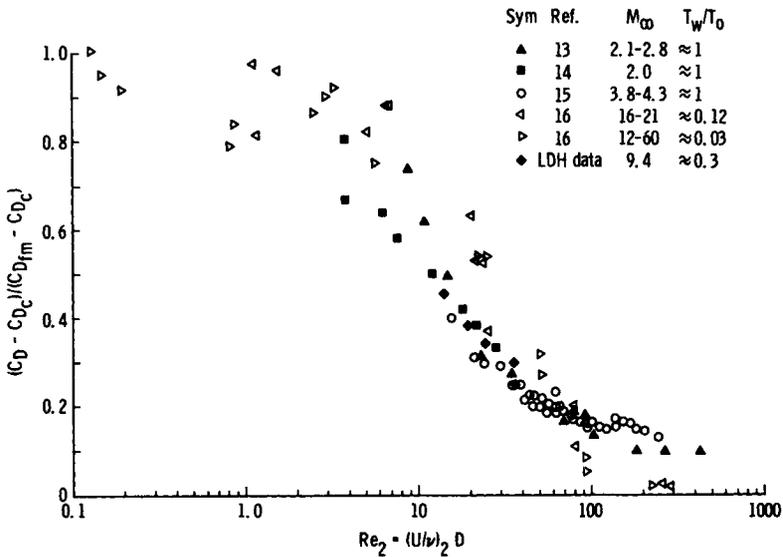
Fig. 16 Comparison of drag coefficients of spheres measured in low density wind tunnels.
