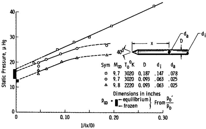
Fig. 6 Approximate determination of static pressure (data have been corrected for temperature gradient along the probe following Ref. 7).
