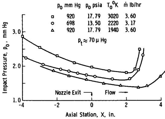
Fig. 10 Axial, centerline impact pressure distributions.
