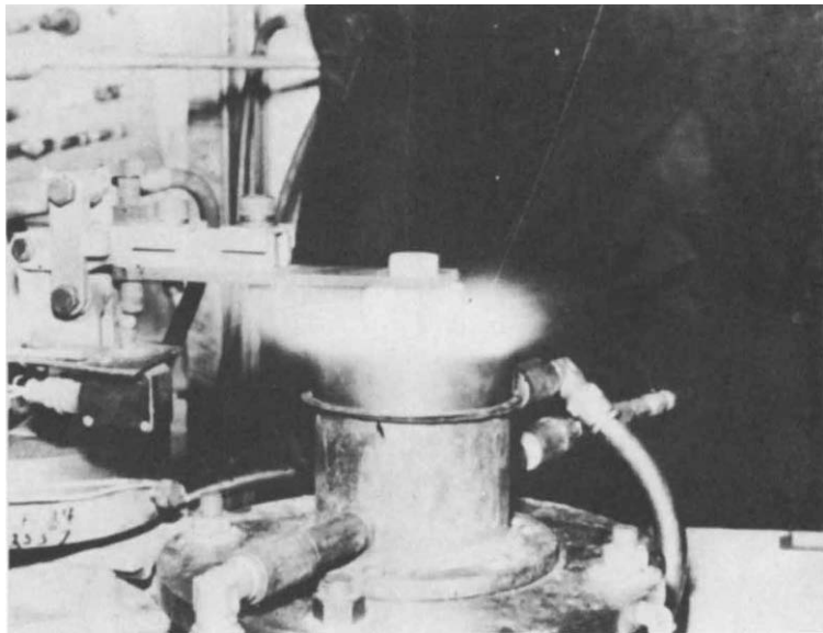
Fig. 5b Ablation test in shroud arc facility.
