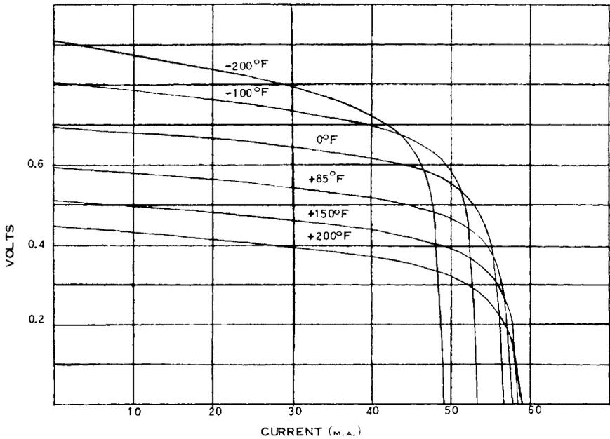
FIG. 4 V-I CURVE vs TEMP. SOLAR CELL CHARACTERISTICS vs TEMP.
