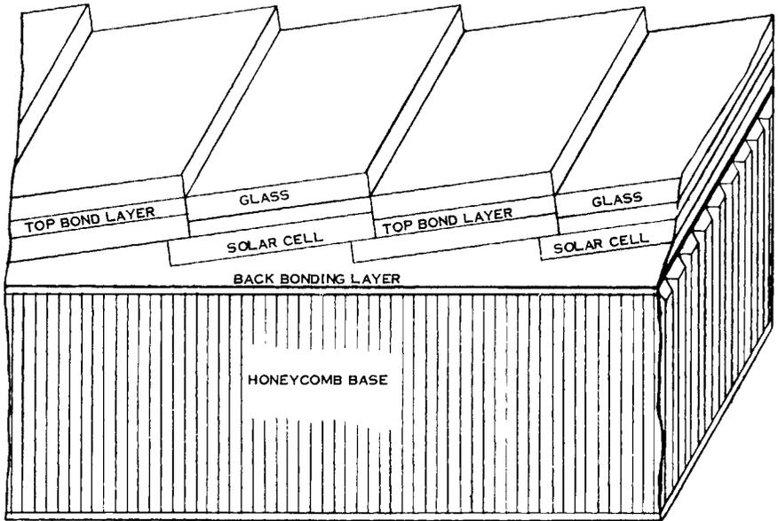
FIG. 3 EXPLODED VIEW OF PADDLE SEGMENT
