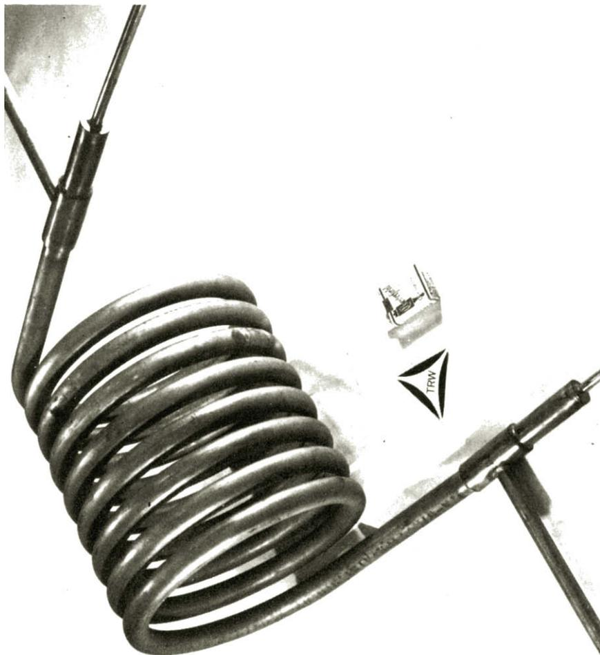
Figure 2. SNAP II Boiler.
