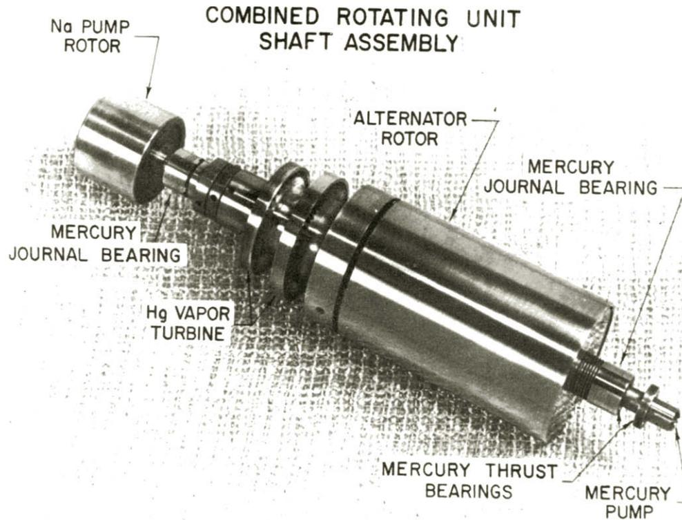
Figure 4. Combined Rotating Unit Shaft Assembly.
