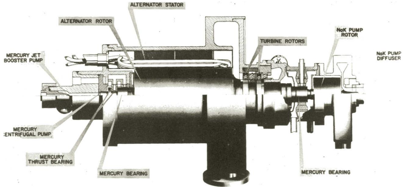
Figure 3. SNAP II Combined Rotating Unit.
