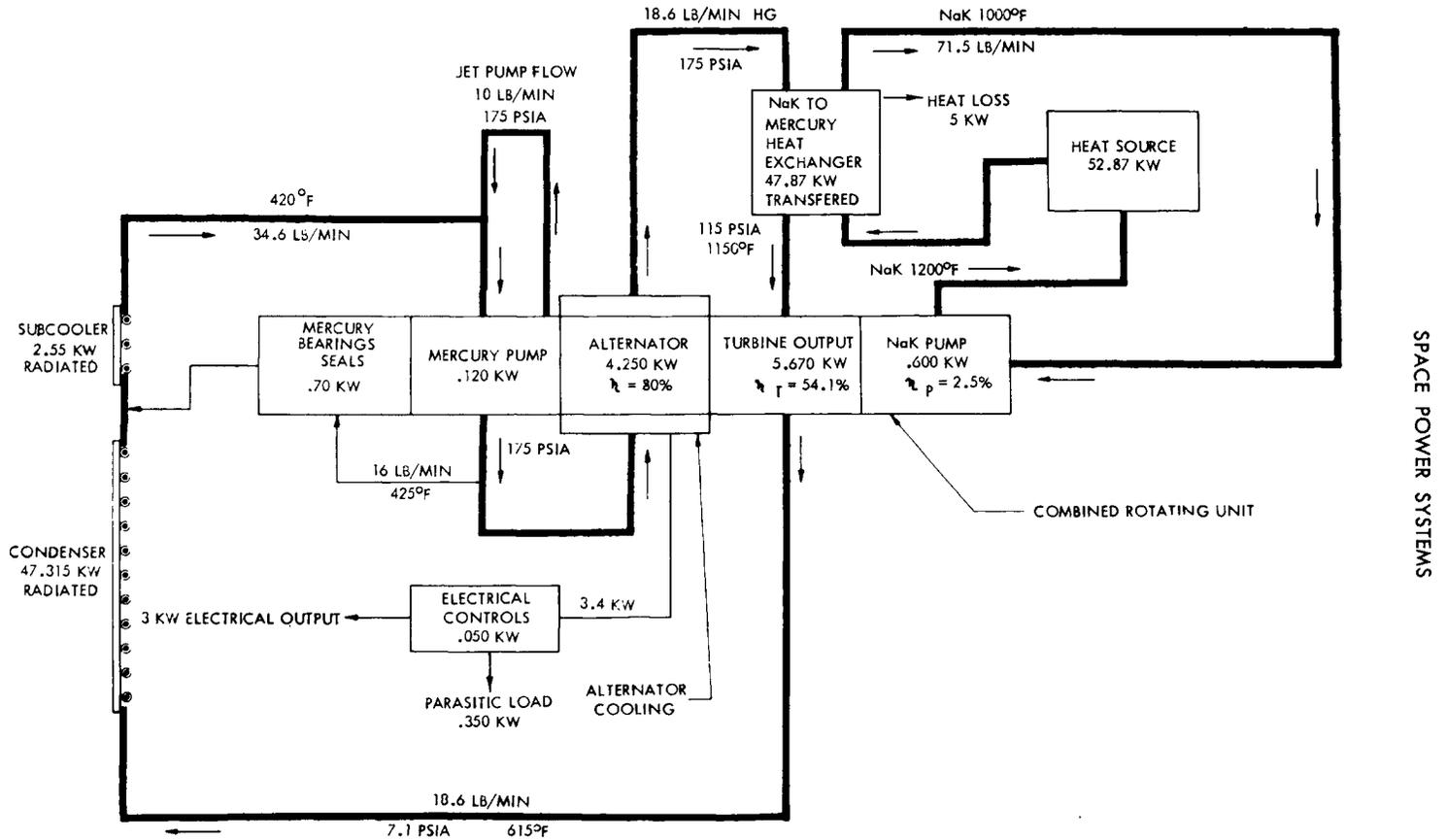
Figure 1. SNAP II Cycle Schematic.
