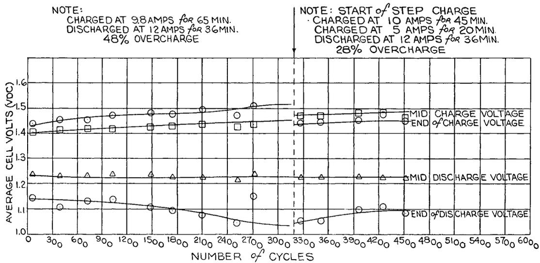
Fig. 7 Orbiting Astronomical Observatory Qualification test. Life cycling data at 90°F
