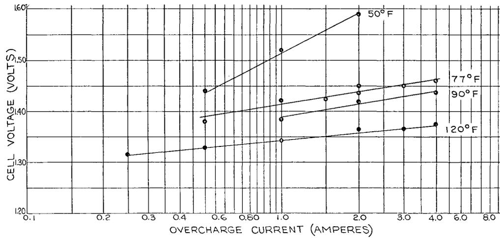
Fig. 5 Overcharge voltage characteristics of VO-20 HS-B hermetically sealed nickel-cadmium cells
