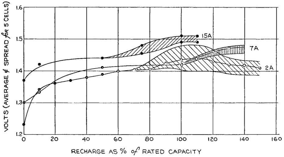
Fig. 3 Charge characteristics of VO-20 HS-B hermetically sealed nickel-cadmium cells at 90°F
