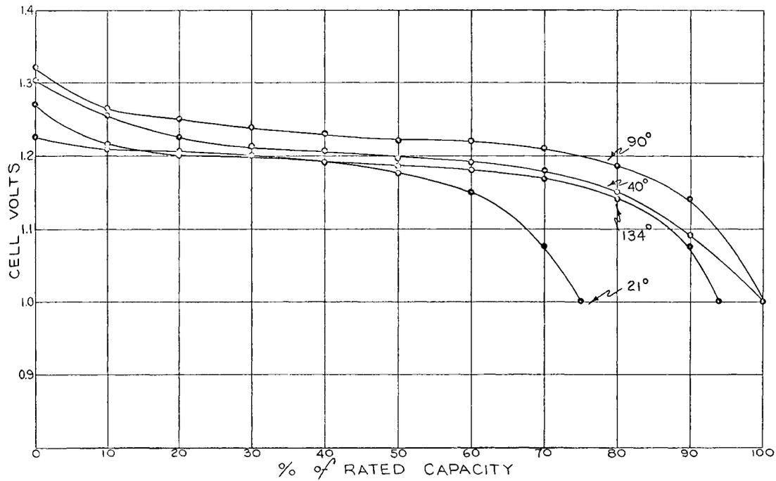
Fig. 2 Discharge characteristics of VO-20 HS-B hermetically sealed nickel-cadmium cells at C/2 rate at various temperatures after 10 amp charge and 8 hr stand
