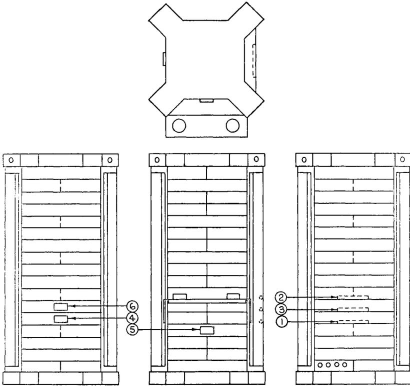
Fig. 11 Orbiting Astronomical Observatory battery assembly.
