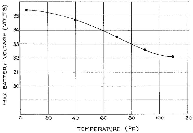
Fig. 9 Maximum limiting charge voltage for a battery of 22 VO-20 HS-B hermetically sealed nickel-cadmium cells
