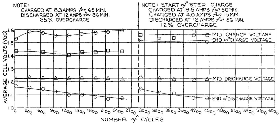
Fig. 6 Orbiting Astronomical Observatory Qualification test.
