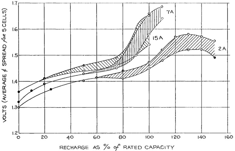
Fig. 4 Charge characteristics of VO-20 HS-B hermetically sealed nickel-cadmium cells at 40°F
