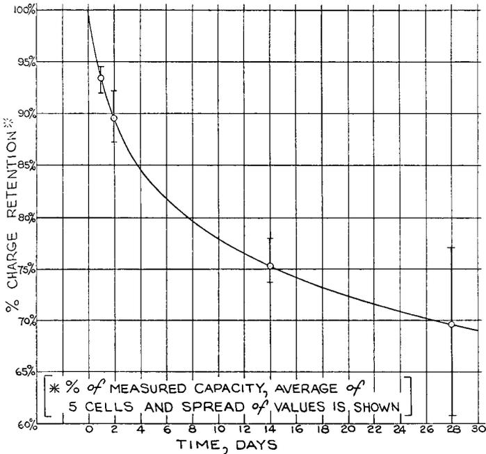
Fig. 10 Charge retention of VO-20 HS-B hermetically sealed nickel-cadmium cells at 90°F
