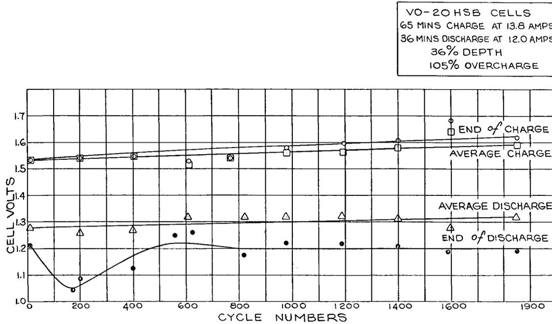
Fig. 8 Orbiting Astronomical Observatory Qualification test.
