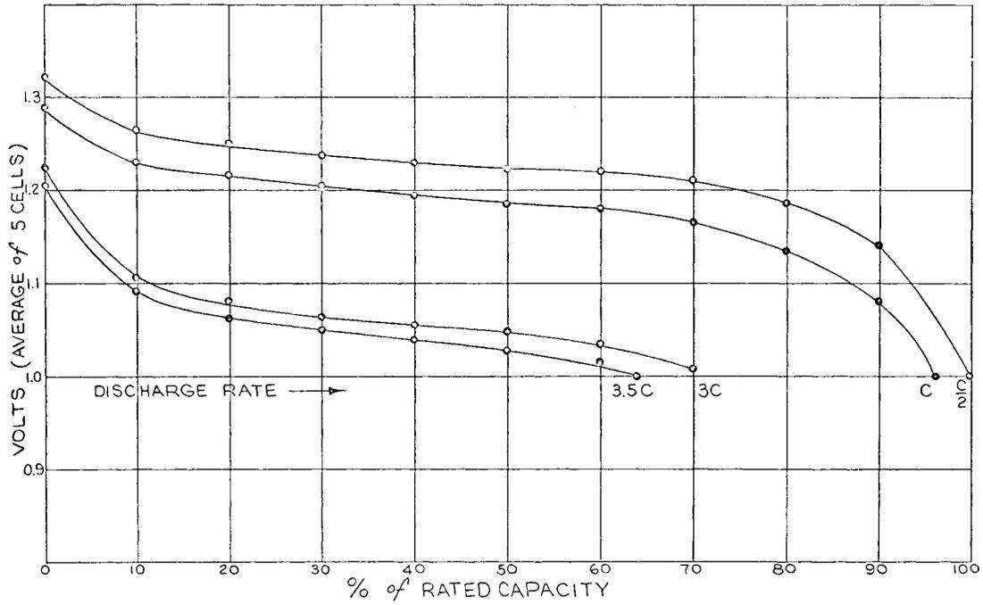
Fig. 1 Discharge characteristics of VO-20 HS-B hermetically sealed nickel-cadmium cells at 90°F
