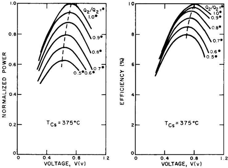
Fig. 14 Normalized power output and efficiency of two diodes in a parallel circuit with power inputs  $Q_1$  and  $Q_2$ . ( $Q_1$  is the power input at  $T_E = 1800^\circ\text{C}$ )
