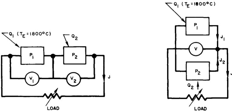
Fig. 11 Circuit diagrams. a) Two diodes in series; b) two diodes in parallel
