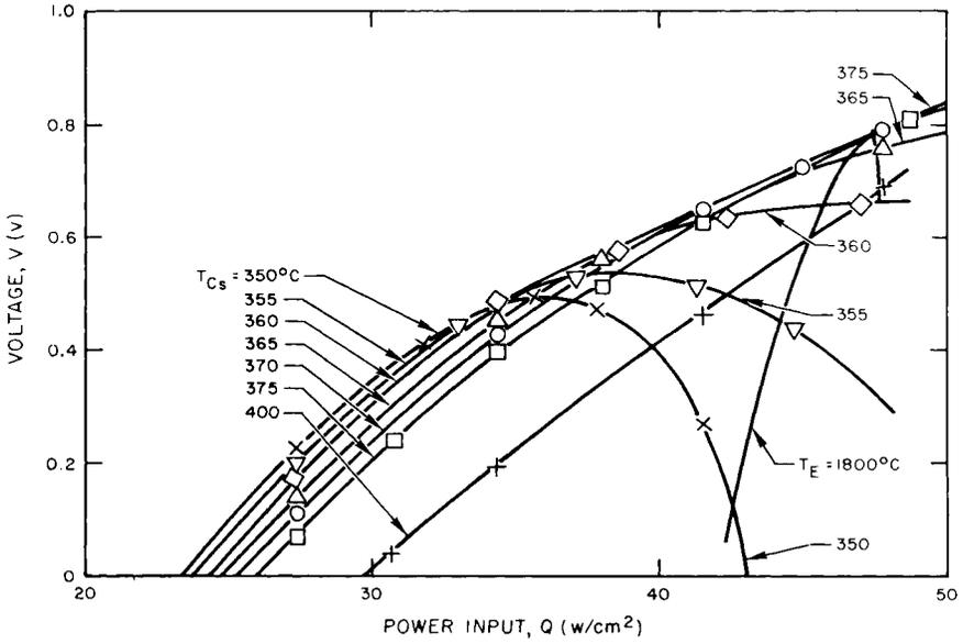
Fig. 6 Voltage vs power input at  $J = 6 \text{ amp/cm}^2$  and  $T_C = 750^\circ\text{C}$
