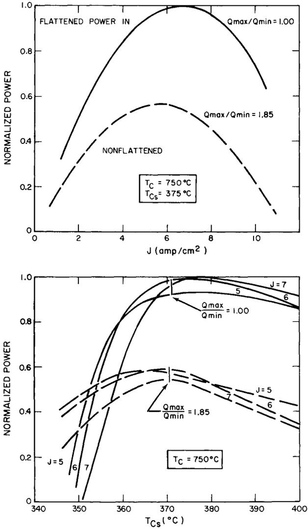
Fig. 18 Normalized power output of a thermionic reactor with 1000 series-connected diodes
