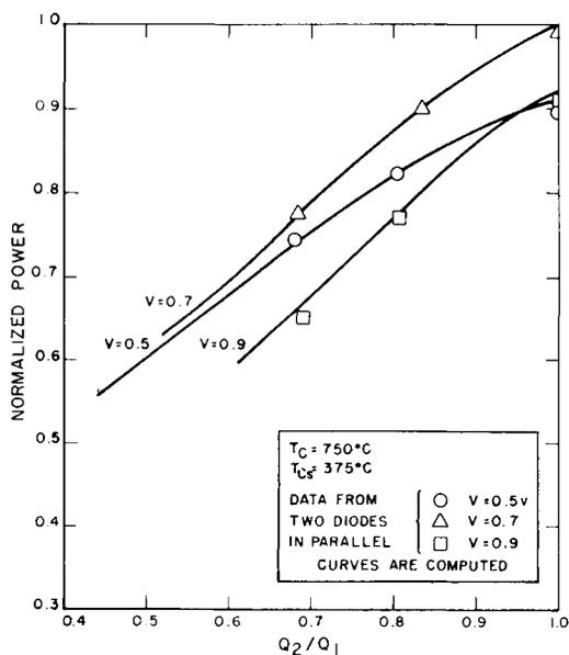
Fig. 17 Operating data for parallel-connected diodes with power inputs  $Q_1$  and  $Q_2$ . ( $Q_1$  is the power input at  $T_E = 1800^\circ\text{C}$ )
