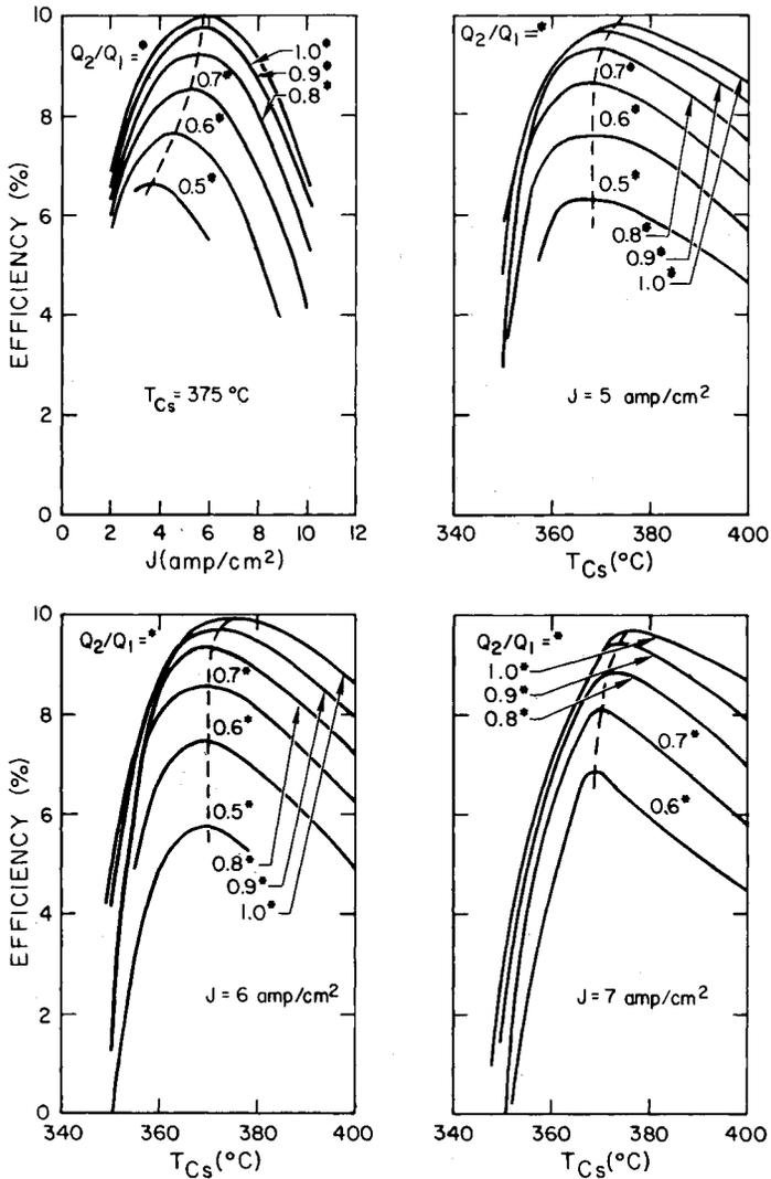
Fig. 13 Efficiency of two diodes in a series circuit with power inputs  $Q_1$  and  $Q_2$ . ( $Q_1$  is the power input at  $T_E = 1800^\circ\text{C}$ )
