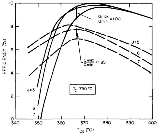
Fig. 19 Efficiency of a thermionic reactor with 1000 series connected diodes
