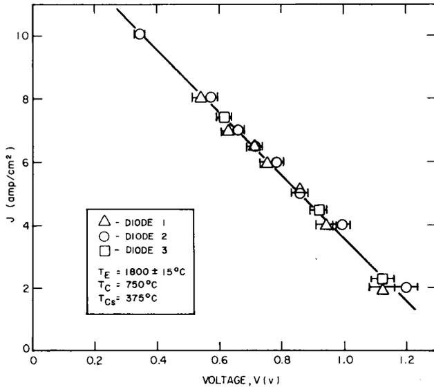
Fig. 9 Comparison of the individual performances of the three diodes at  $T_E = 1800 \pm 15^{\circ}C$
