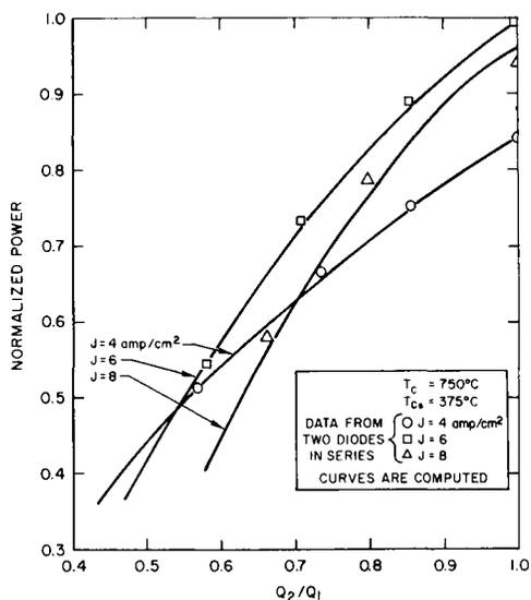
Fig. 16 Operating data for series-connected diodes with power inputs  $Q_1$  and  $Q_2$ . ( $Q_1$  is the power input at  $T_E = 1800^\circ\text{C}$ )
