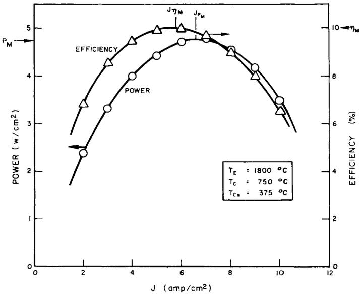
Fig. 3 Maximization of power and efficiency and the optimum values of  $J$
