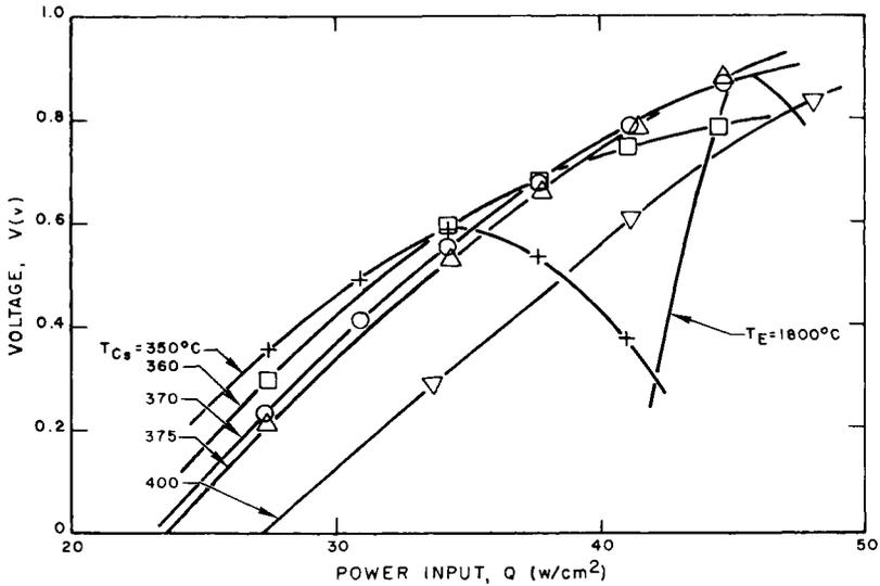
Fig. 5 Voltage vs power input at  $J=5 \text{ amp/cm}^2$  and  $T_C = 750^\circ\text{C}$
