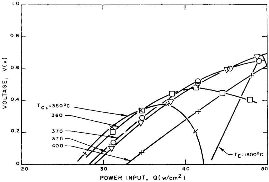
Fig. 7 Voltage vs power input at  $J = 7 \text{ amp/cm}^2$  and  $T_C = 750^\circ\text{C}$
