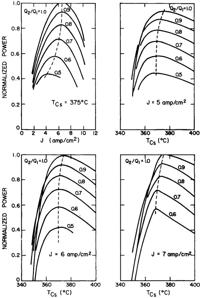
Fig. 12 Normalized power output of two diodes in a series circuit with power inputs  $Q_1$  and  $Q_2$ . ( $Q_1$  is the power input at  $T_E = 1800^\circ\text{C}$ )
