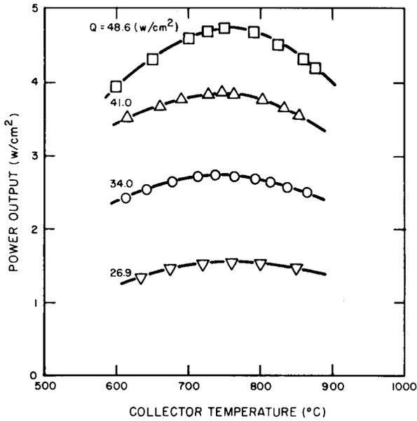
Fig. 8 Effect of collector temperature on power output at  $T_{Cs} = 375^{\circ}C$
