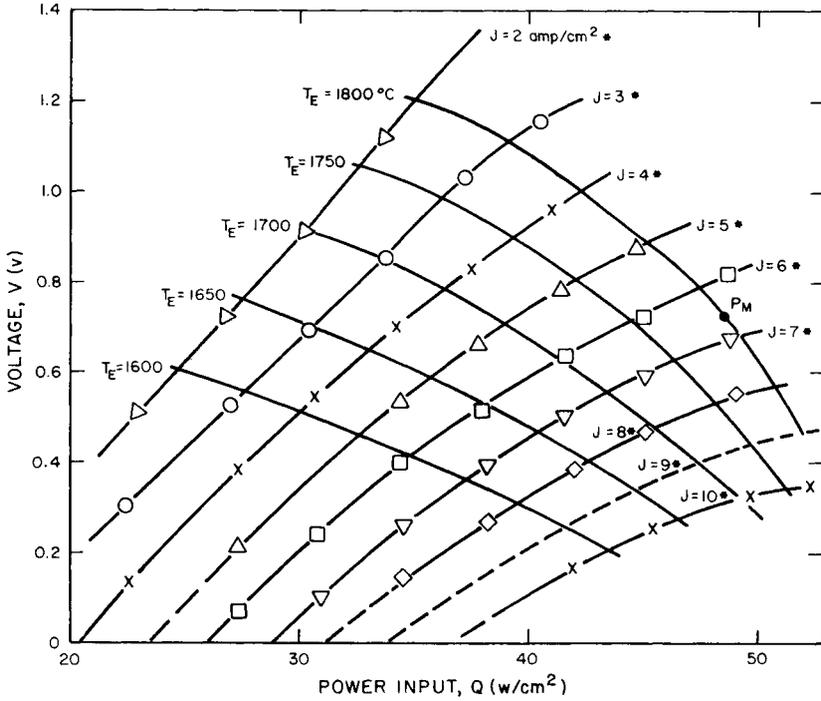
Fig. 4 Voltage vs power input at  $T_C = 750^\circ\text{C}$  and  $T_{CS} = 375^\circ\text{C}$
