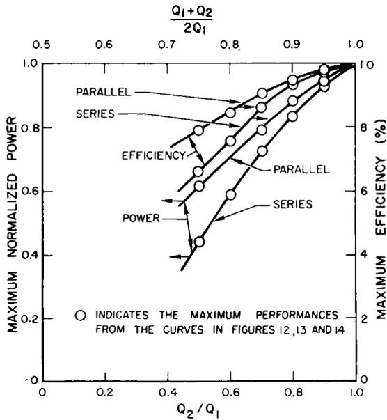
Fig. 15 Maximized power and efficiency of two diodes in series and parallel circuits vs  $Q_2/Q_1$
