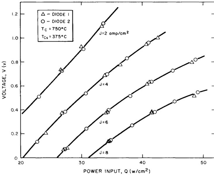
Fig. 10 Comparison of diodes 1 and 2 at  $T_{CS} = 375^\circ\text{C}$  and  $T_C = 750^\circ\text{C}$ . (These two diodes are tested in series and parallel circuits)
