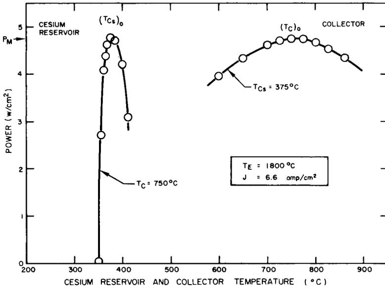
Fig. 2 Optimization of cesium reservoir and collector temperature
