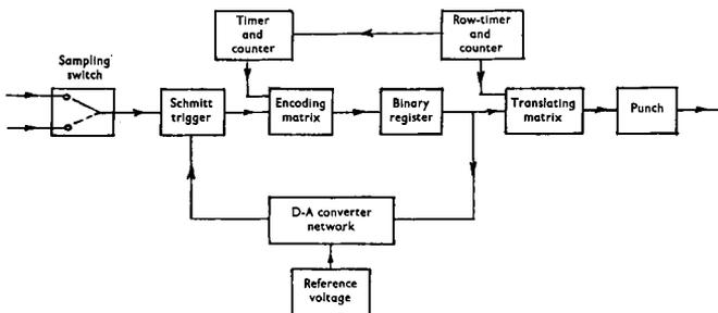
Fig. 4.—Simplified diagram of the analog-digital converter.
