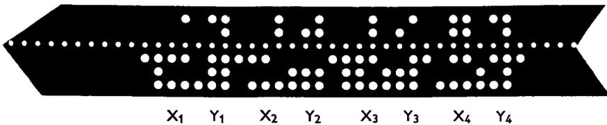
Fig. 5.—Punched tape pattern.
