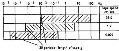
Fig. 3.—Frequency range of magnetic tape unit.
